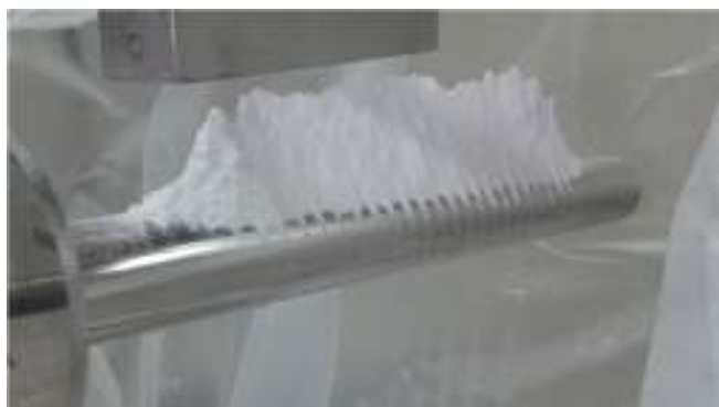
Fig.4-1 State of powder deposited on the upper surface of the bar magnet.
