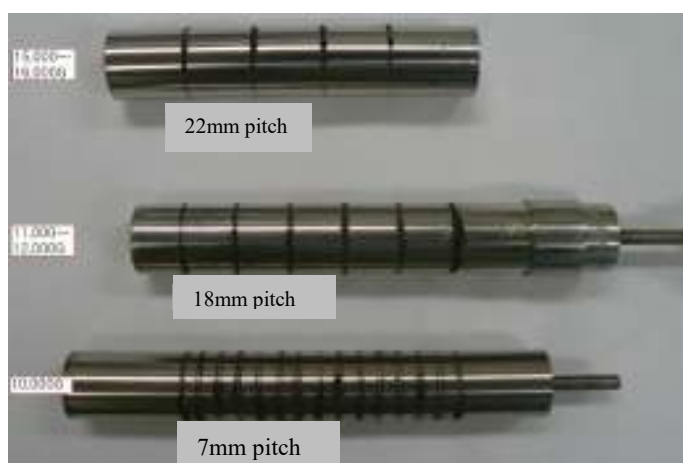
Fig.1-5 Examples of magnetic pole spacing and magnetic flux density of bar magnets.
