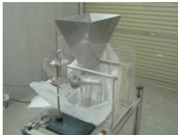
Fig.4-3 Bar magnet tilt angle testing equipment.
