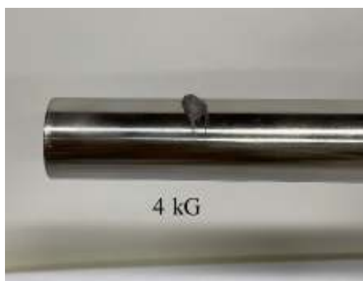
Fig.6-2 0.2g of SUS wear powder is all absorbed by 4kG.
