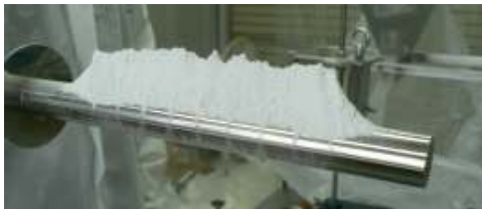
Fig.4-6 Powder (Silica S) that continues to cover the top surface of the bar magnet ( \theta = 0^\circ )
