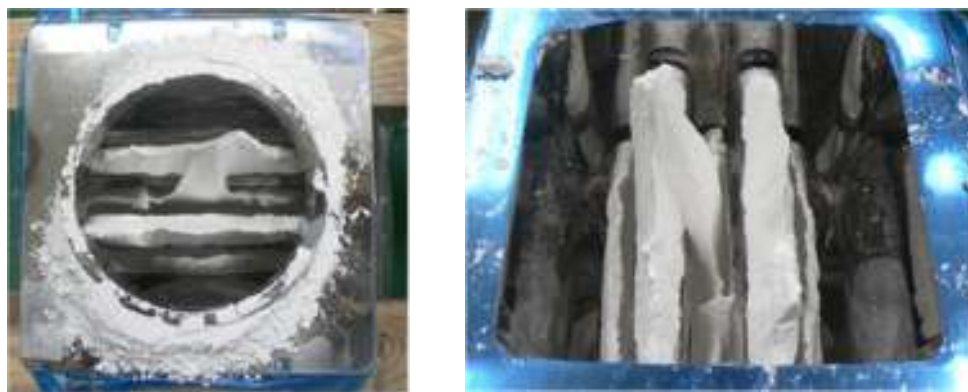
Fig.5-1 Powder bridge between bar magnets.
