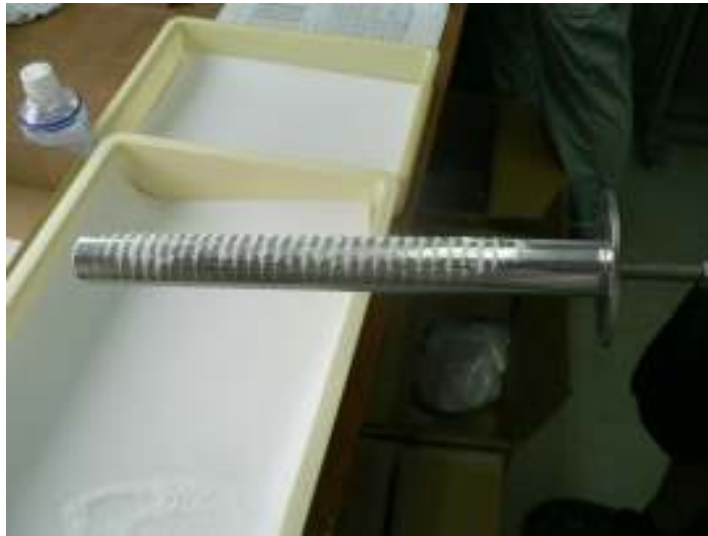
Fig.3-3 Magnetic particles captured by a bar magnet.
