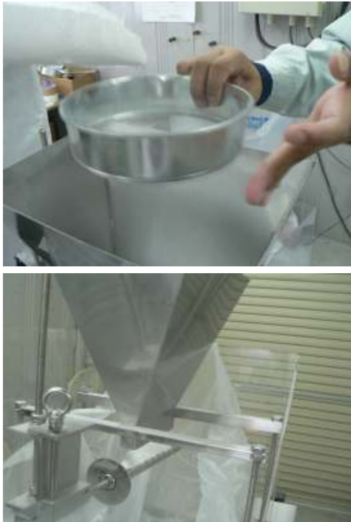
Fig.3-2 Inserting silica powder by hand sieving.
