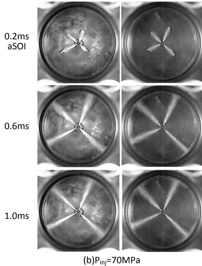
Fig.5-5 Rapeseed spray development of rapeseed oil with different injection pressure and different volume-sac nozzle ( $T_i=298\text{K}$ )
