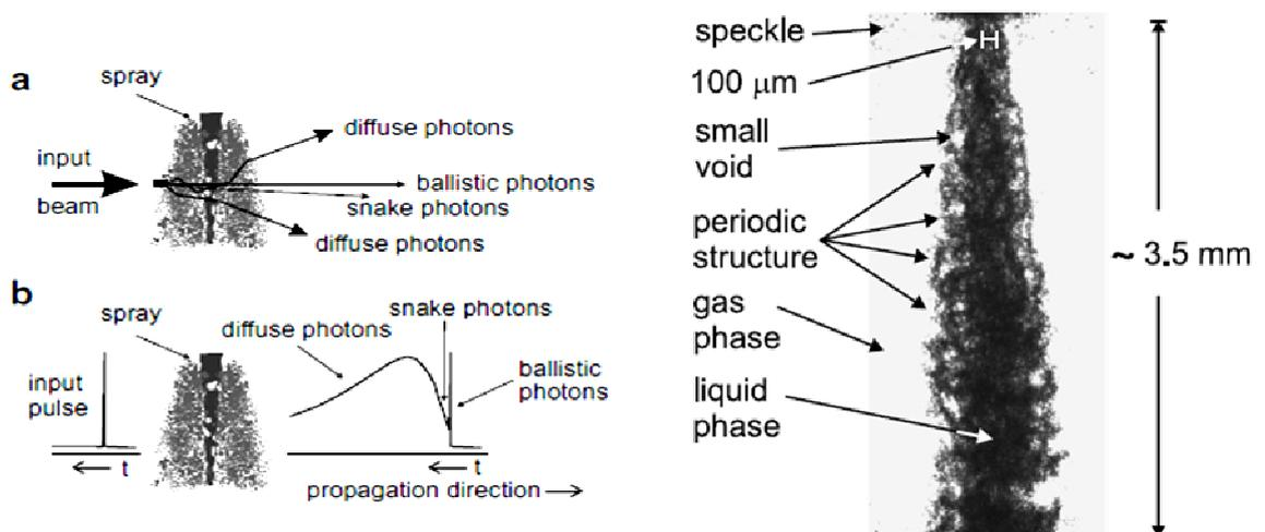
Fig.2-3 Schematic of ballistic, snake and diffuse photon.
