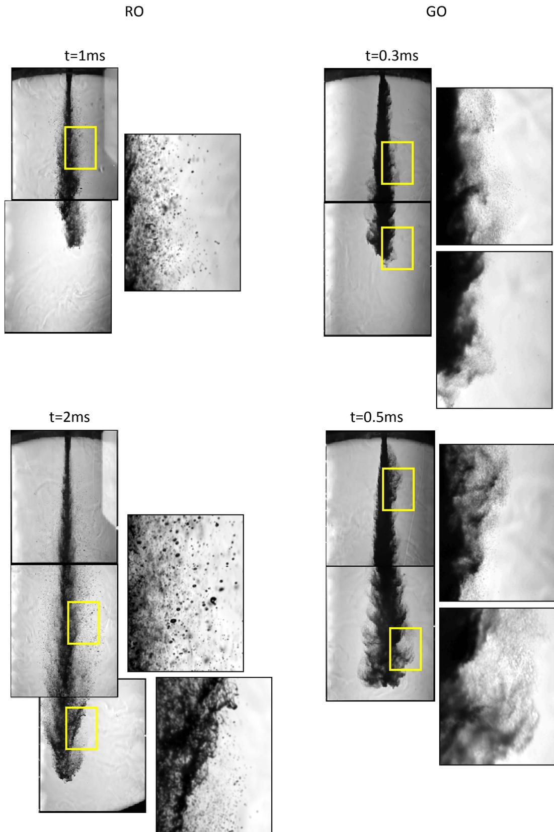
Fig.7-4 Comparison between rapeseed oil to gas oil spray development (IDI nozzle,  $P_{inj}=40\text{MPa}$ ,  $T_i=700\text{K}$ )
