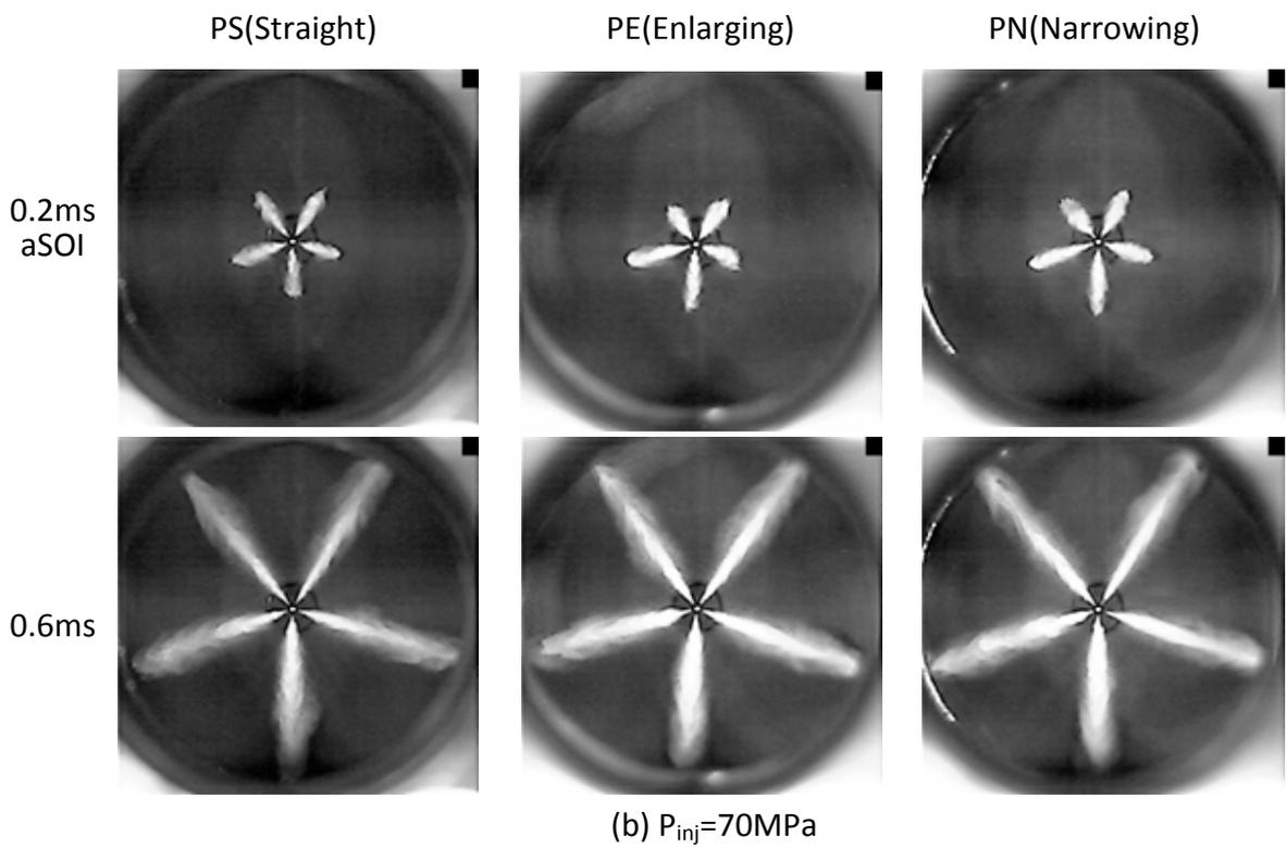
Fig.5-8 Rapeseed oil spray developments of three types of nozzle hole configuration
