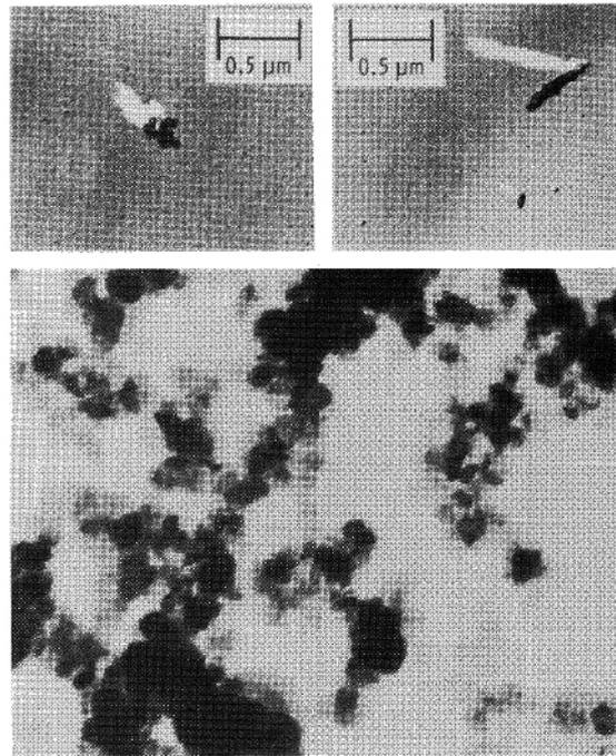
Fig.1-3 Photomicrograph of diesel particulate; cluster (upper left), chain (upper right), collection from filter (lower)[10]
