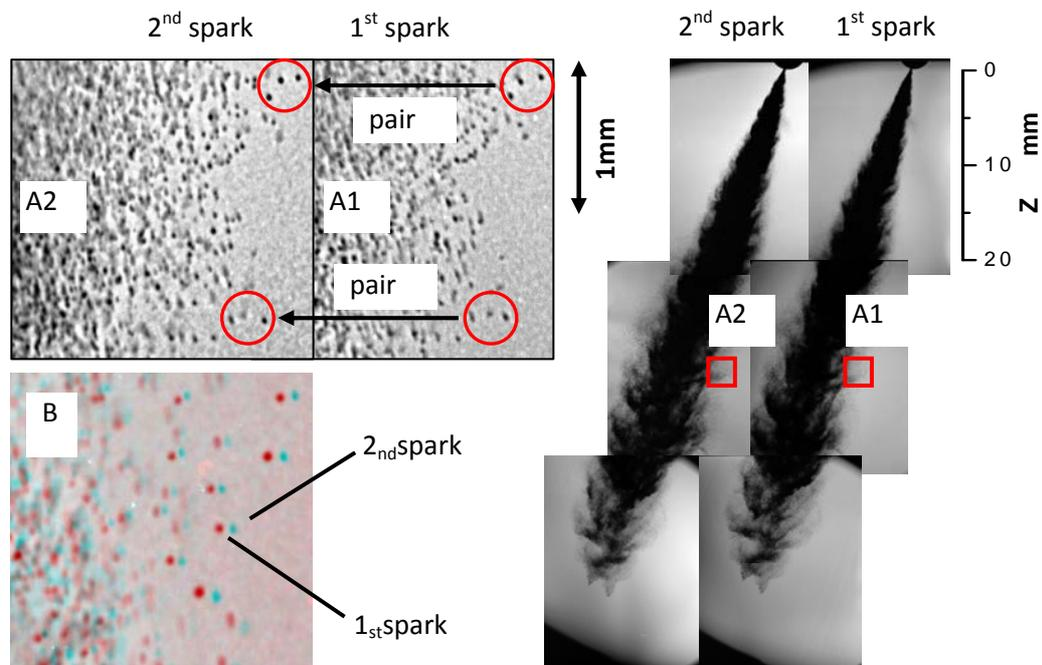
Fig.2-18 Dual nano spark images of non-evaporating spray ( $T_i=298\text{K}$ ,  $P_{inj}=40\text{MPa}$ ,  $t=0.5\text{ms}$ ,  $\Delta t=15\mu\text{s}$ )
