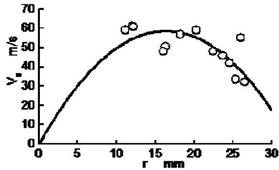
(a) Swirl speed distribution measured from center during injection
