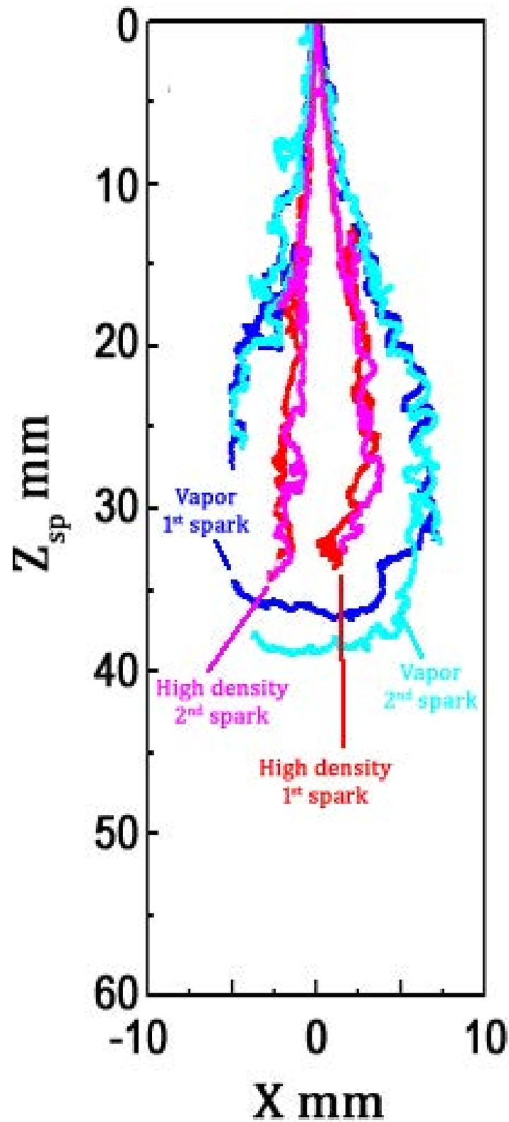
Fig.4-9 Progression of high density region and vapor boundary in gas oil spray ( $T_i=700K$ ,  $P_{inj}=70MPa$ ,  $\Delta t=25\mu s$ ,  $t=0.50ms$ )
