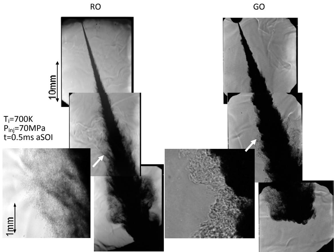
Fig.4-4 Comparison of spray structure and droplets between rape-seed oil and gas oil sprays ( $T_i=700K$ ,  $P_{inj}=70MPa$ )
