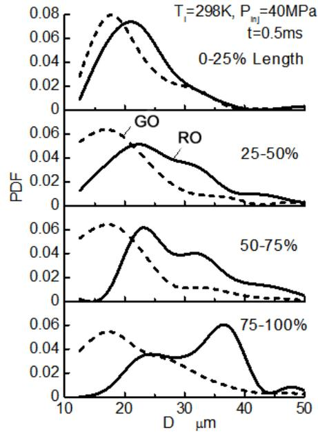
Fig.4-5 Comparison of droplets distribution between rape-seed oil and gas oil sprays ( $T_i=298\text{K}$ ,  $P_{inj}=40\text{MPa}$ )
