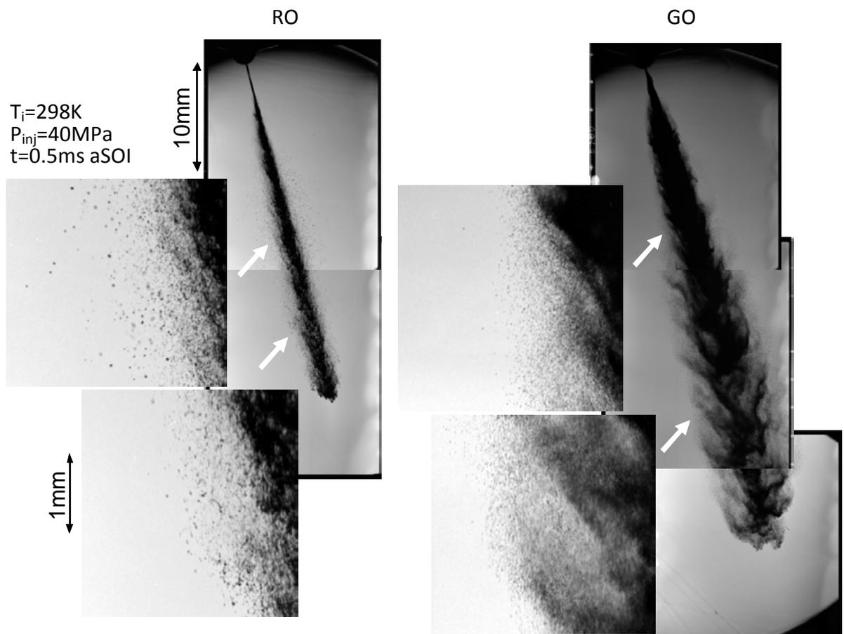
Fig.4-1 Comparison of spray structure and droplets between rape-seed oil and gas oil sprays ( $T_i=298K$ ,  $P_{inj}=40MPa$ )
