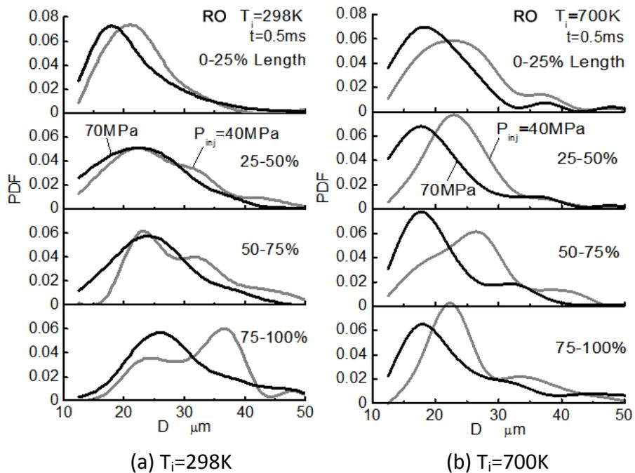
Fig.4-6 Effect of injection pressure on droplets size distribution of rapeseed oil spray
