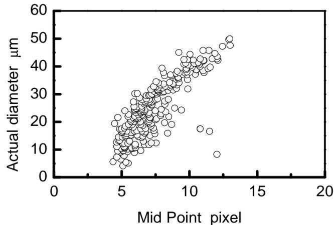
Fig.3-9 Correlation between Mid Point and actual diameter of particles filtered by *Ratio\_IN*, *Ratio\_OUT*, and *prdev*
