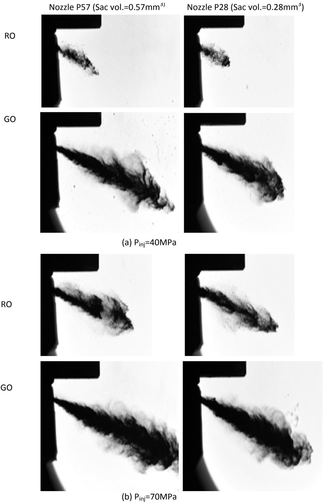
Fig.5-7 Effect of nozzle sac-volume on spray structure at initial stage of injection (t=0.5ms aSOI)
