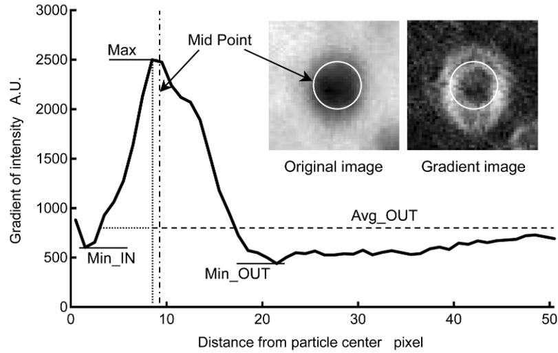
Fig.3-4 Details of intensity gradient profiles
