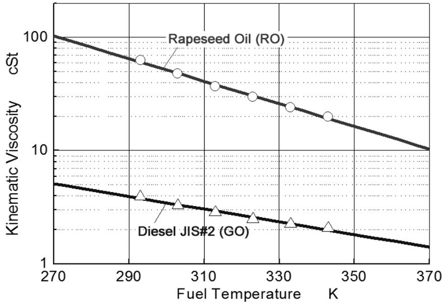
Fig.2-12 Effect of fuel temperature on fuel kinematic viscosity
