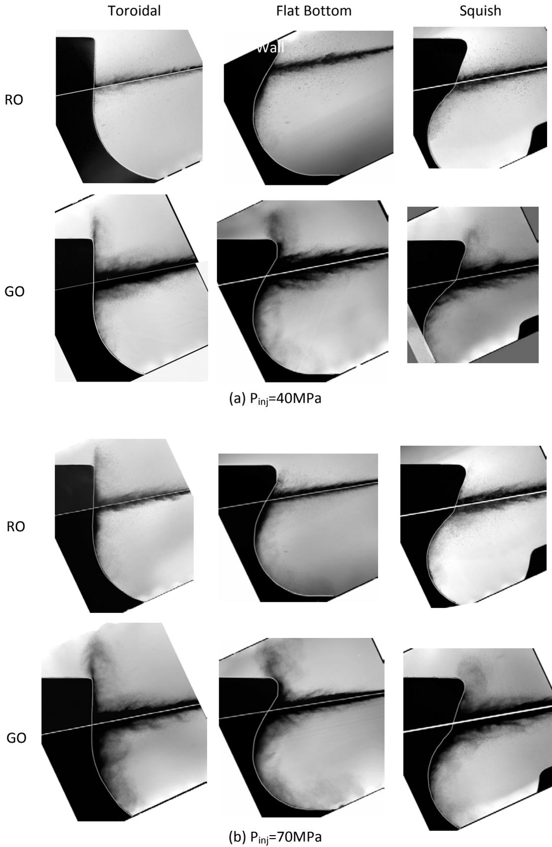
Fig.6-2 Wall impingement spray comparison between rapeseed oil and gas oil ( $T_i=298\text{K}$ , 0.5ms after impingement)
