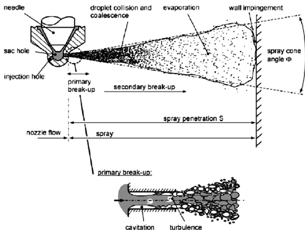
Fig.1-6 Schematic of full cone spray[39]
