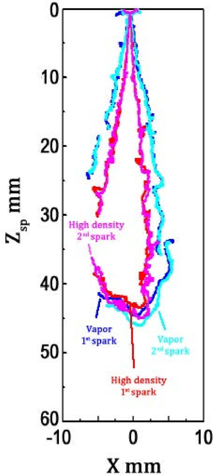
Fig.4-8 Progression of high density region and vapor boundary in gas oil spray
