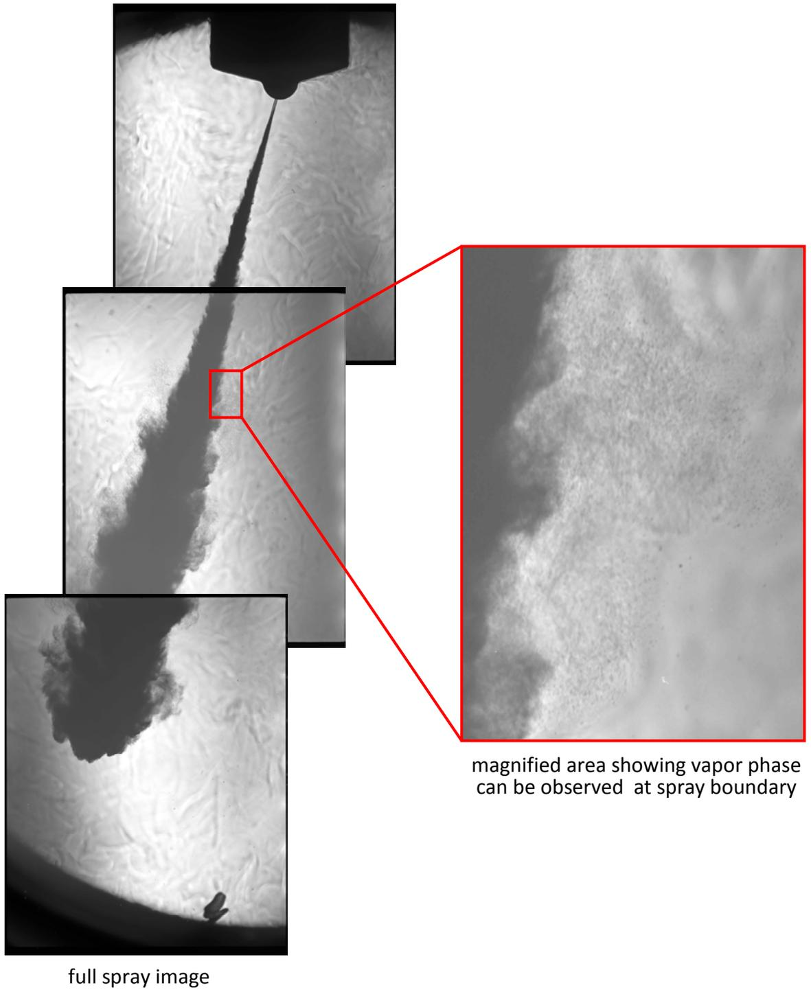
Fig.4-12 Vaporization of rapeseed oil spray ( $T_i=850K$ ,  $P_{inj}=70MPa$ ,  $t=0.50ms$ )
