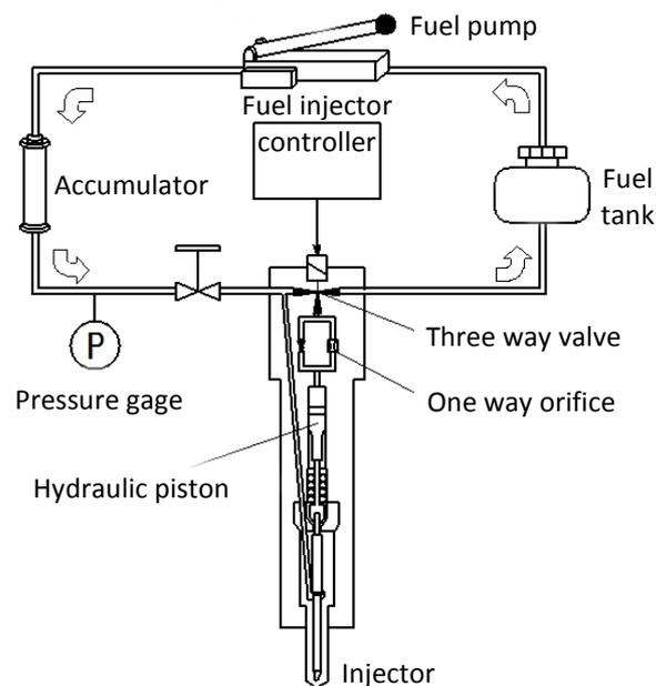
Fig.2-8 High pressure fuel injection system
