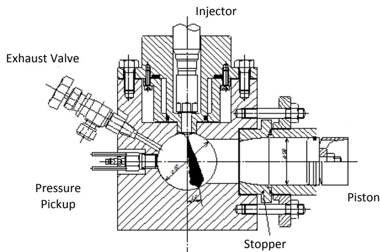
Fig.2-7 Cross section of spray chamber (nano spark)
