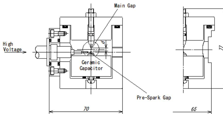
Fig.2-9 Cross section of spark head
