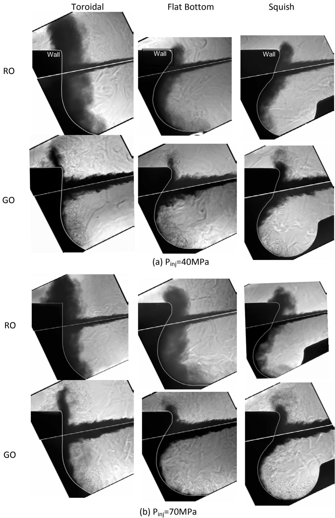
Fig.6-4 Wall impingement spray comparison between rapeseed oil and gas oil ( $T_i=700\text{K}$ , 0.5ms after impingement)
