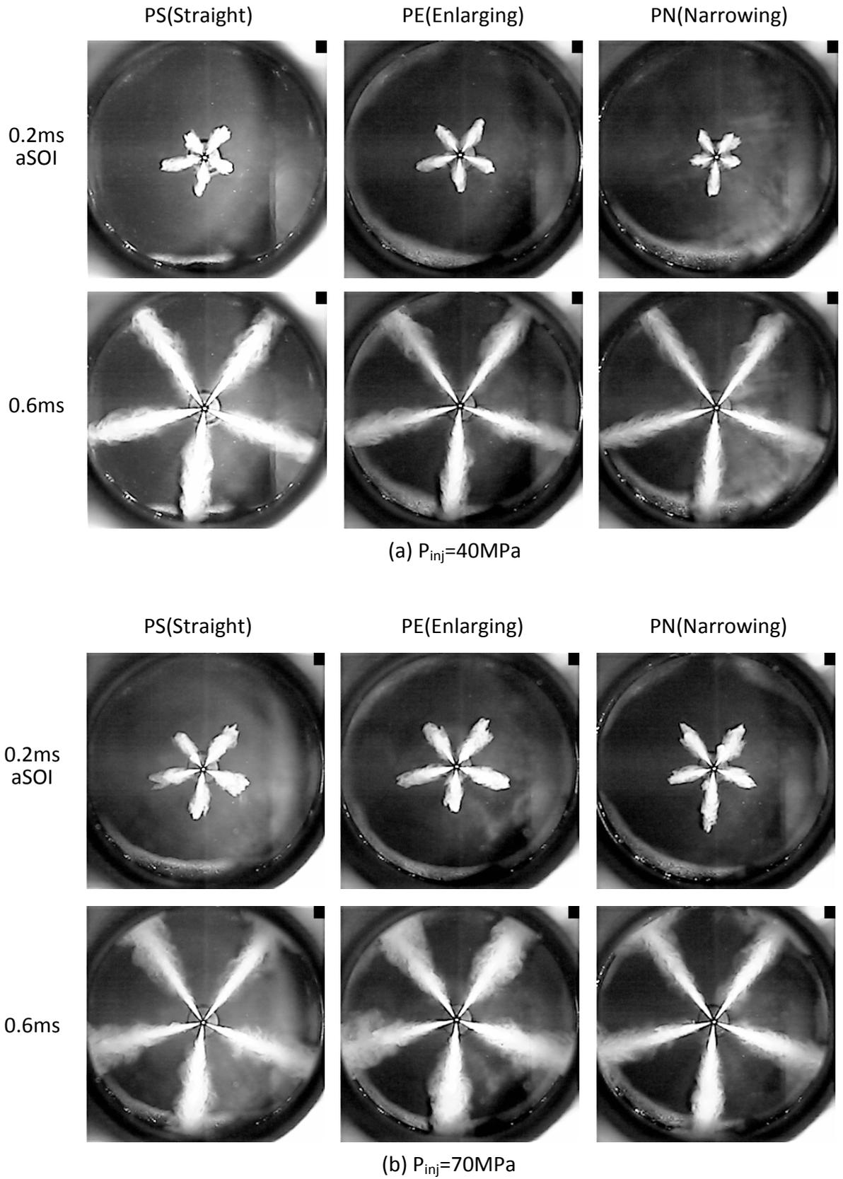
Fig.5-10 Gas oil spray developments of three types of nozzle hole configuration
