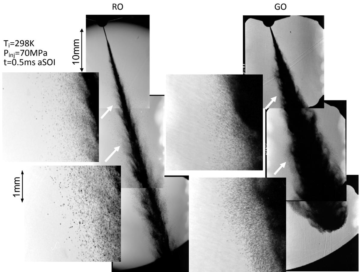
Fig.4-2 Comparison of spray structure and droplets between rape-seed oil and gas oil sprays ( $T_i=298K$ ,  $P_{inj}=70MPa$ )
