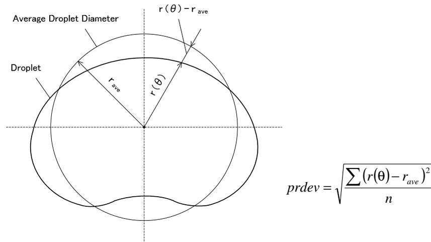
Fig.3-6 Schematic deviation of particle radius
