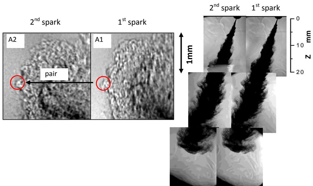
Fig.2-19 Dual nano spark images of evaporating spray ( $T_i=700\text{K}$ ,  $P_{inj}=70\text{MPa}$ ,  $t=0.5\text{ms}$ ,  $\Delta t=15\mu\text{s}$ )
