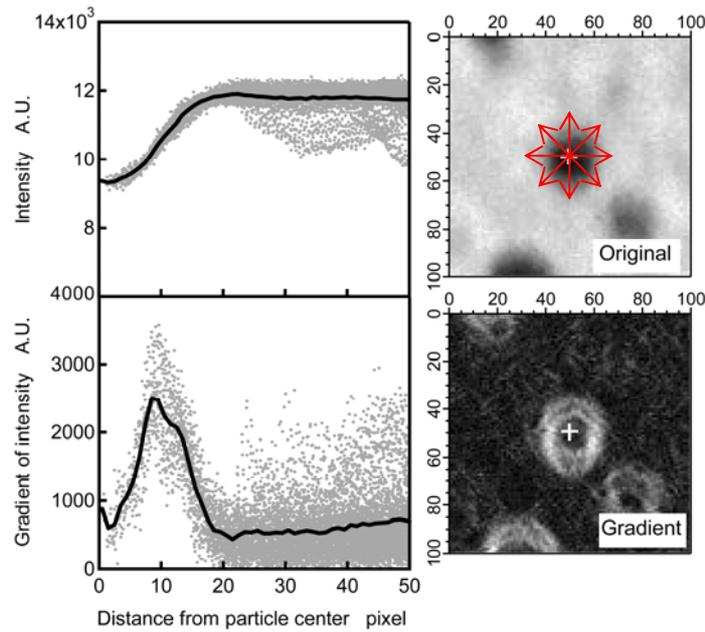
Fig.3-3 Intensity and gradient intensity profiles
