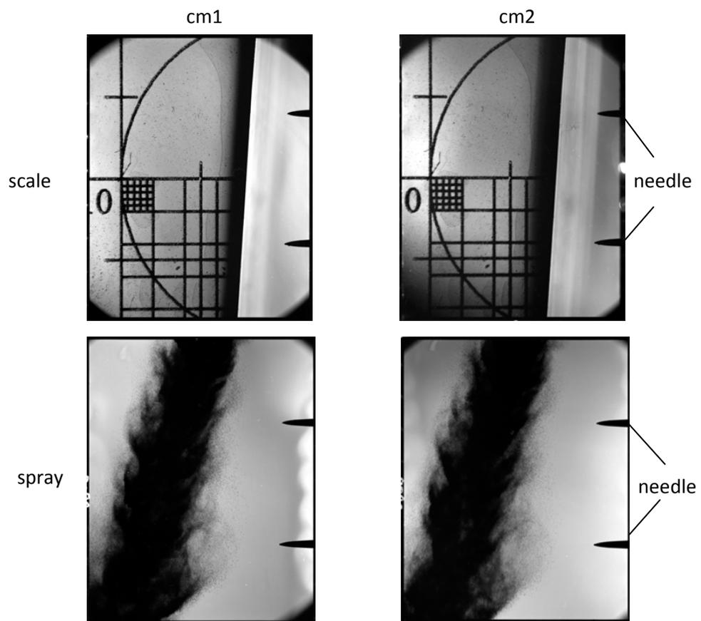
Fig.3-14 Reference needle in scale and spray image for camera 1 and camera 2
