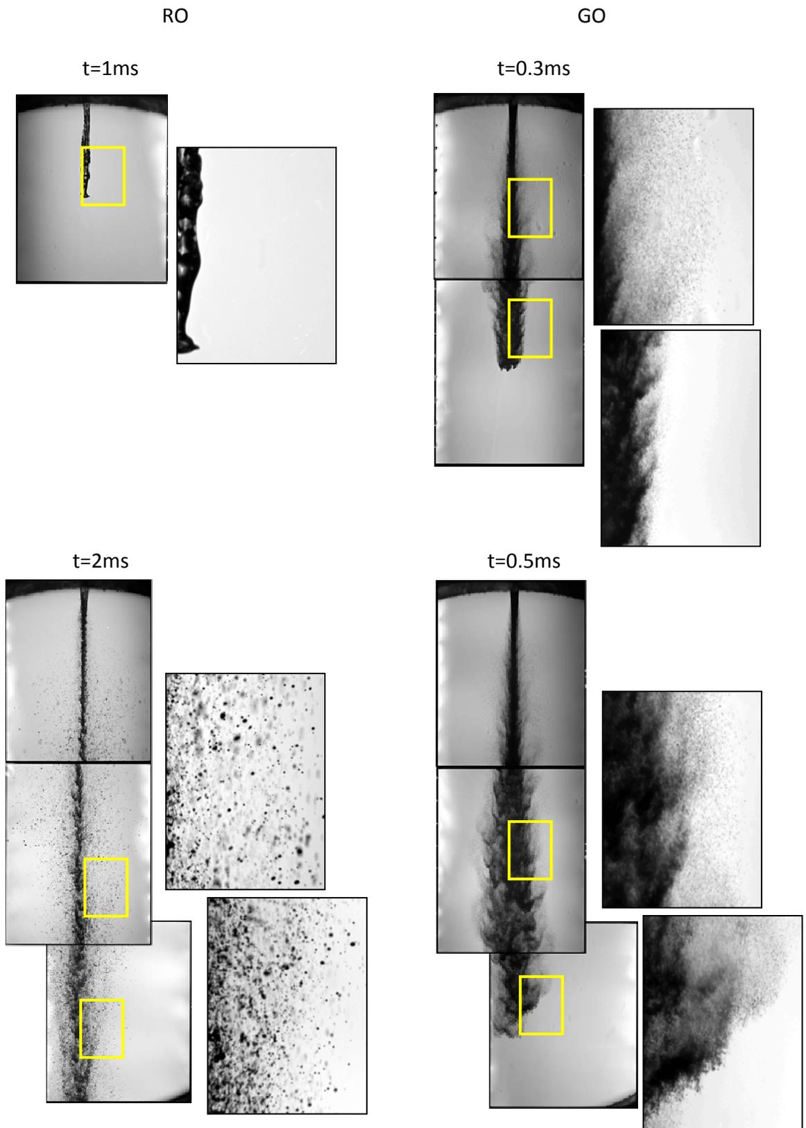
Fig.7-3 Comparison between rapeseed oil to gas oil spray development (IDI nozzle,  $P_{inj}=40\text{MPa}$ ,  $T_i=298\text{K}$ )
