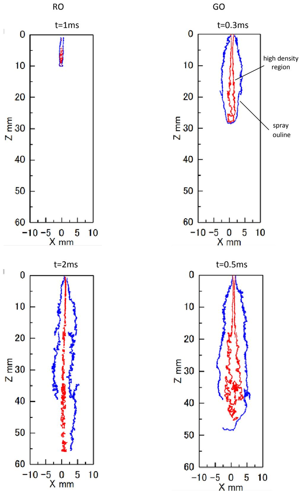
Fig.7-5 Spray development outline and progression of liquid core in IDI nozzle ( $P_{inj}=40\text{MPa}$ ,  $T_i=298\text{K}$ )
