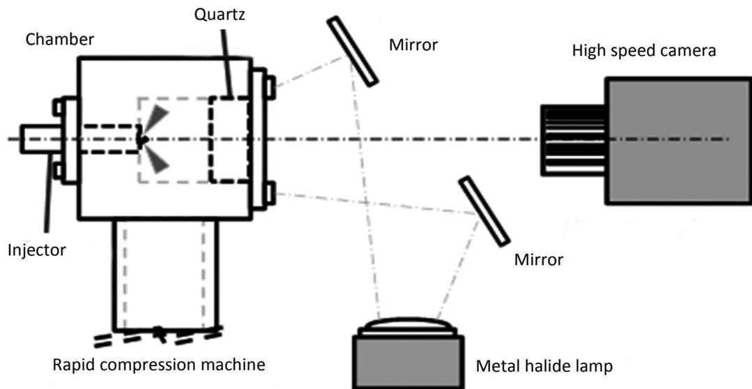
Fig.2-6 Schematic diagram of high-speed camera direct imaging method
