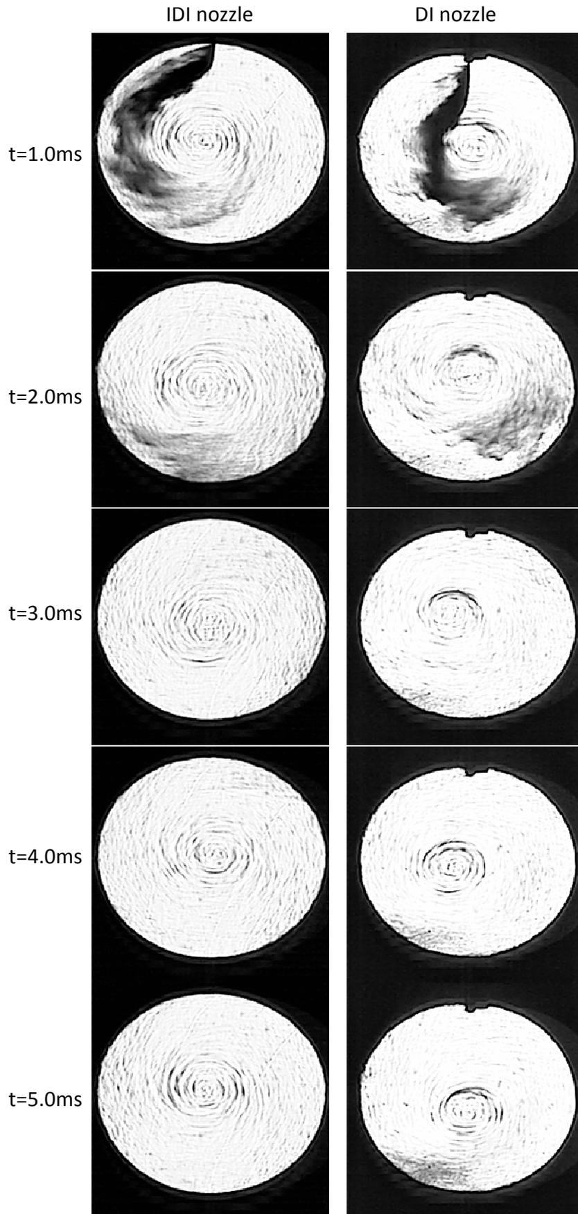
Fig.7-11 Comparison between IDI nozzle and DI nozzle gas oil spray development under swirl influence ( $P_{inj}=40\text{MPa}$ ,  $T_i=700\text{K}$ )
