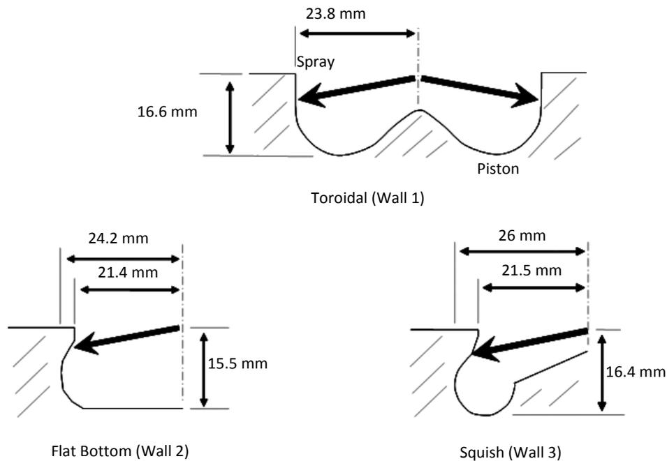
Fig.6-1 Geometry of impinging wall
