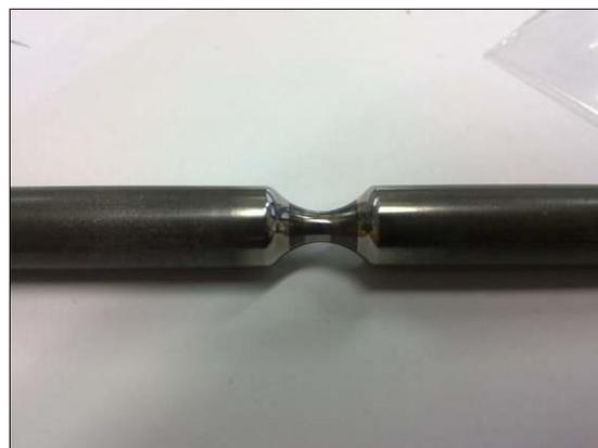
Figure 2-9 Specimen after UNSM treatment.
