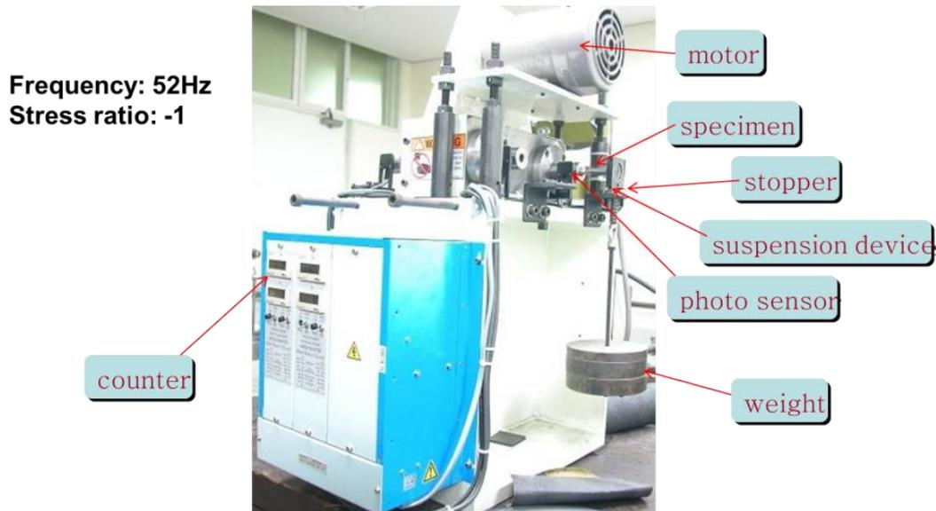
Figure 2-12 Rotating-bending fatigue test machine
