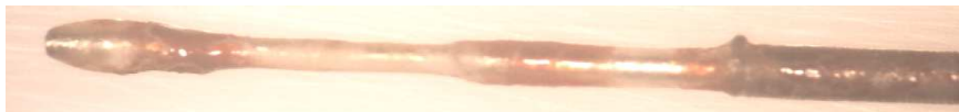
Fig. 6-4 Photograph of glucose sensor with PU/PDMS-outer membrane after 7 days implantation in blood vessel.
