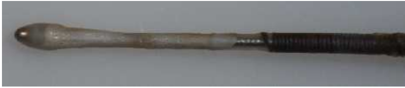
Fig. 7-11 Photograph of heparin/urokinase-coated glucose sensor after 10 days implantation in blood vessel.
