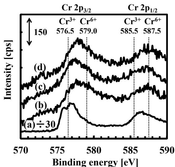
**Fig. 7** XPS spectra of (a) crystalline  $\alpha$ -Cr<sub>2</sub>O<sub>3</sub>, and 1.8 wt% Cr-MCM-41 (b) before ODH of isobutane, (c) after the pretreatment with O<sub>2</sub> flow and (d) after ODH of isobutane
