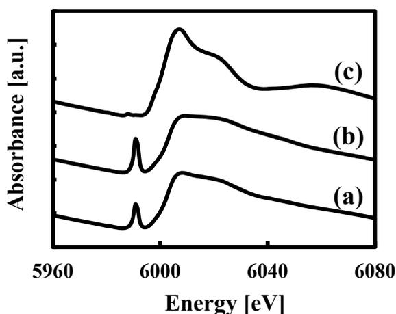
**Fig. 8** Cr K-edge XANES spectra of (a) 2.2 wt% Cr-MCM-41 (a) before ODH of isobutane, (b) after the pretreatment with  $\text{O}_2$  flow and (c) after ODH
