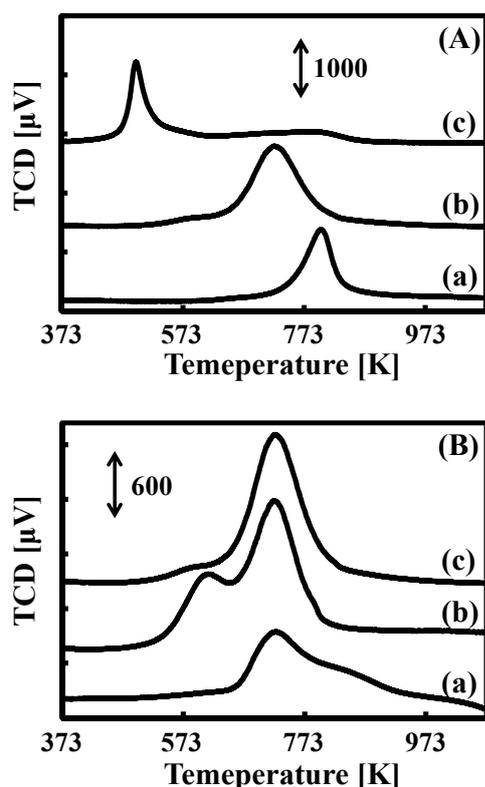
**Fig. 6** TPR spectra of (A) (a) 1.8 wt% V-MCM-41, (b) 1.8 wt% Cr-MCM-41 and (c) 2.2 wt% Cu-MCM-41, and (B) (a) crystalline  $\alpha$ -Cr<sub>2</sub>O<sub>3</sub> (b) 1.8 wt% Cr-MCM-41 without the pretreatment and (c) 1.8 wt% Cr-MCM-41 with the pretreatment
