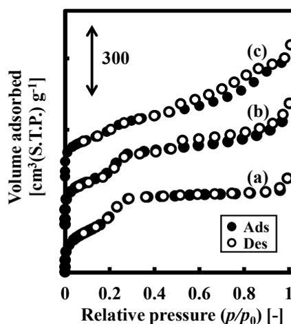
Fig. 2 N<sub>2</sub> adsorption-desorption isotherms of (a) MCM-41, (b) 1.8 wt% Cr-MCM-41 and (c) 2.7 wt% Fe-MCM-41 (The starting point of each isotherm is different)
