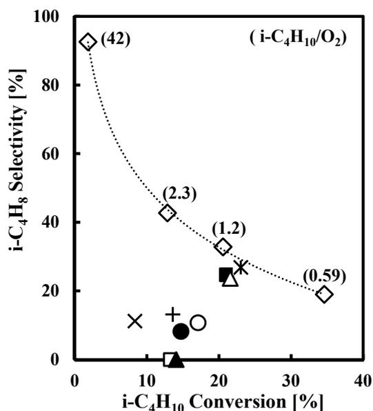
**Fig. 5** Isobutene selectivity versus isobutane conversion of 1.8 wt% Cr-MCM-41 ( $\diamond$ ) at different  $i\text{-C}_4\text{H}_{10}/\text{O}_2$  ratios (0.59, 1.2, 2.3, or 42), M-MCM-41 (M = V ( $\circ$ ), Mn ( $\bullet$ ), Fe ( $\square$ ), Co ( $\blacksquare$ ), Ni ( $\triangle$ ), Cu ( $\blacktriangle$ ), and Mo ( $*$ )), MCM-41 ( $\times$ ), and  $\alpha\text{-Cr}_2\text{O}_3$  ( $+$ ) at  $i\text{-C}_4\text{H}_{10}/\text{O}_2$  ratio = 1.2, 723 K, and 6.0 h on-stream
