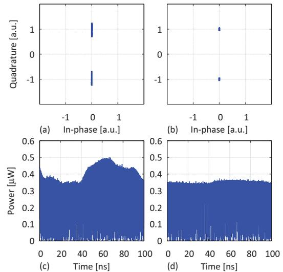
Fig. 13. Examples of (a)(b) constellations and (c)(d) waveforms of the converted quadrature BPSK signal on  $x$ -polarization when phase-locking between signal and pumps is (b)(d) activated and (a)(c) not activated.
