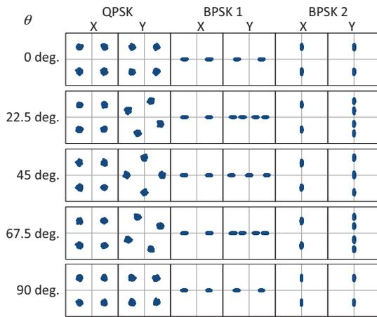
Fig. 9. Constellation diagrams of the original QPSK signal and the converted two BPSK signals at  $\theta = 0, 22.5, 45, 67.5$  and  $90$  degrees.
