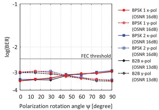
Fig. 11. BER as a function of polarization rotation angle  $\psi$  with 3-dB PDL on the vertical axis.
