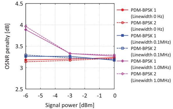
Fig. 8. OSNR penalty from B2B at BER on the FEC threshold as a function of signal power with linewidth as a parameter.
