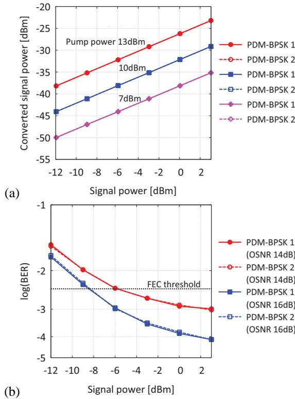
Fig. 4. Simulated results showing (a) converted PDM-BPSK signal power as a function of original PDM-QPSK signal power with pump power as a parameter and (b) BER as a function of original PDM-QPSK signal power with OSNR as a parameter.
