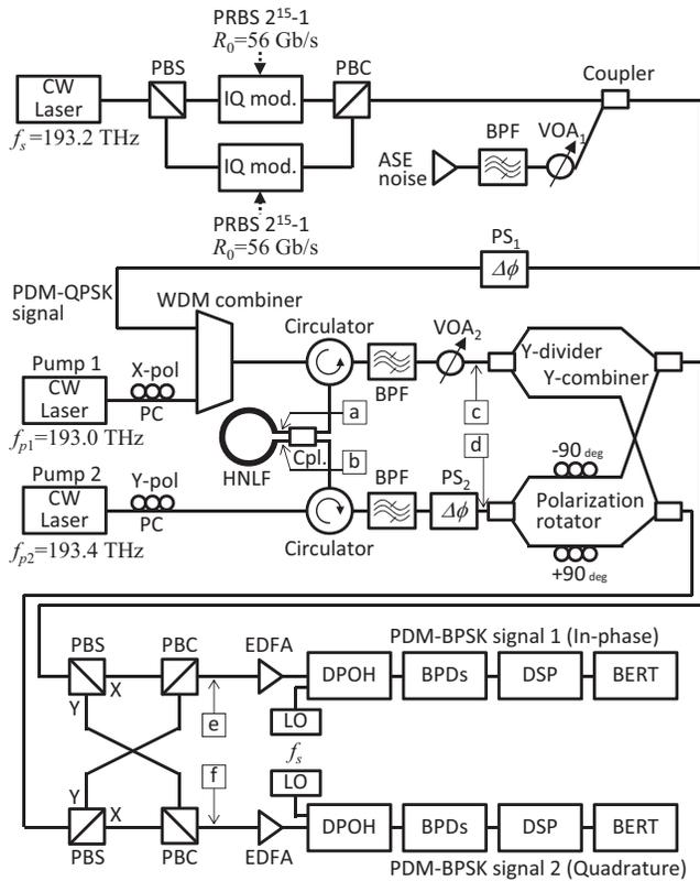
Fig. 2. Setup used in numerical simulation.
