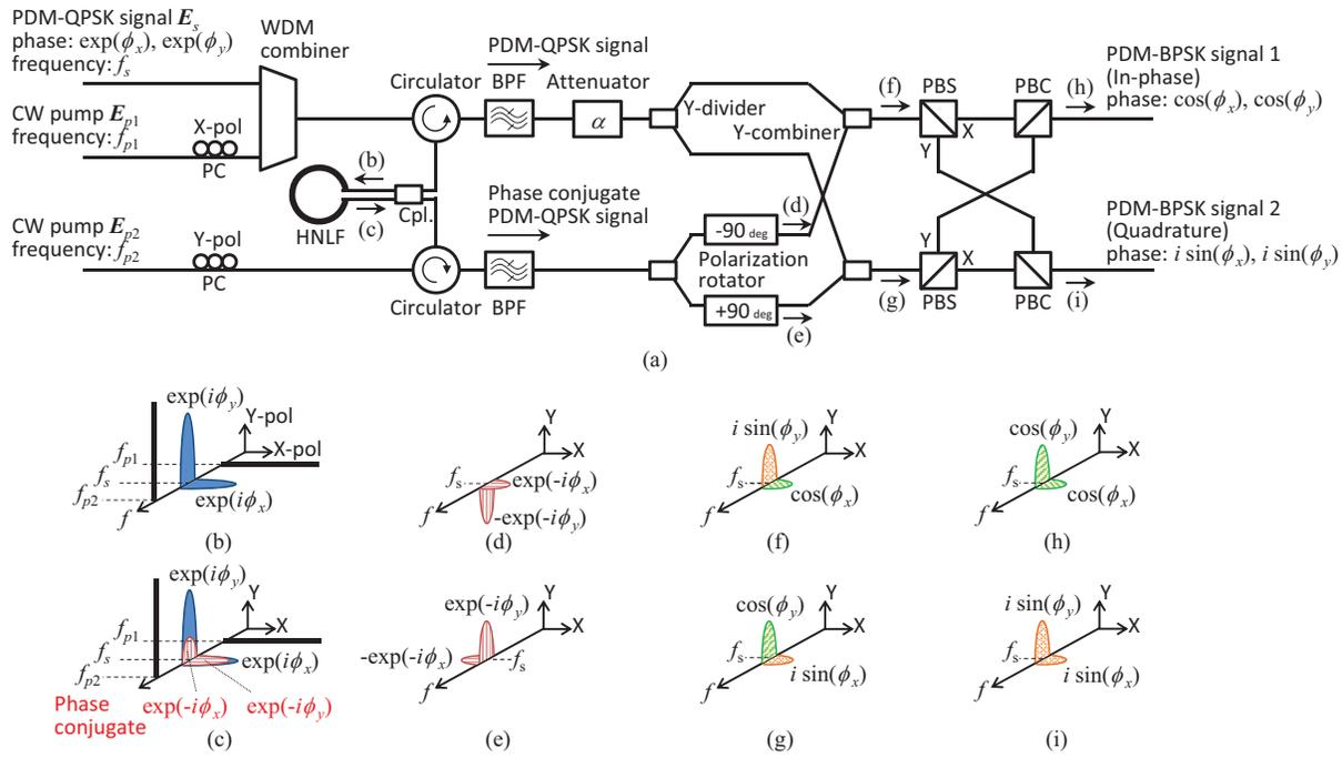
Fig. 1. Schematic diagram of the proposed all-optical wavelength preserved modulation format conversion from PDM-QPSK to PDM-BPSK, (a) system configuration and (b)-(f) signal spectra at each point indicated in (a).
