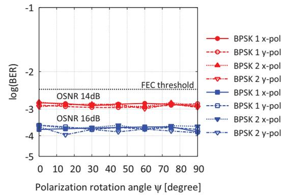
Fig. 7. BER as a function of polarization rotation angle  $\psi$  with OSNR as a parameter.
