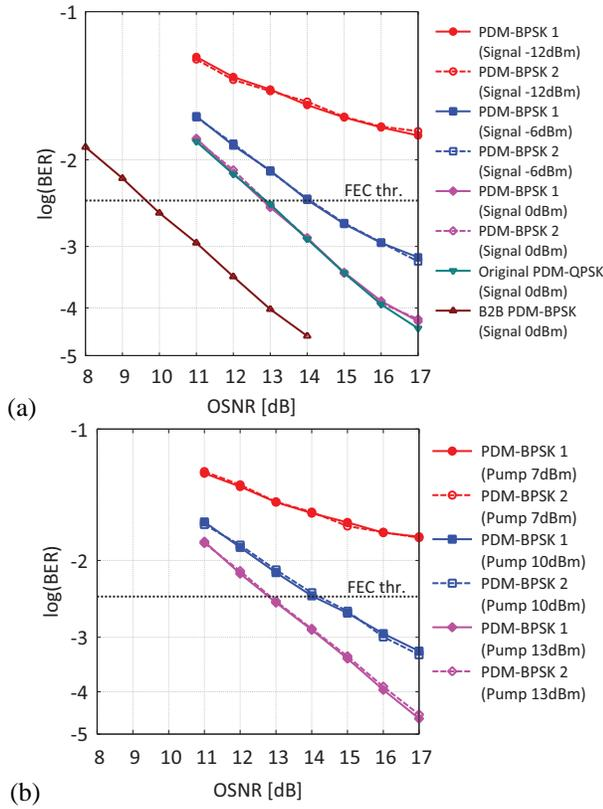
Fig. 6. BER as a function of OSNR with (a) signal power and (b) pump power as parameters.
