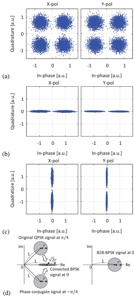
Fig. 5. Constellation map of (a) the original PDM-QPSK signal and the converted (b) in-phase and (c) quadrature PDM-BPSK signals, and (d) schematic of the phase-to-amplitude noise conversion.
