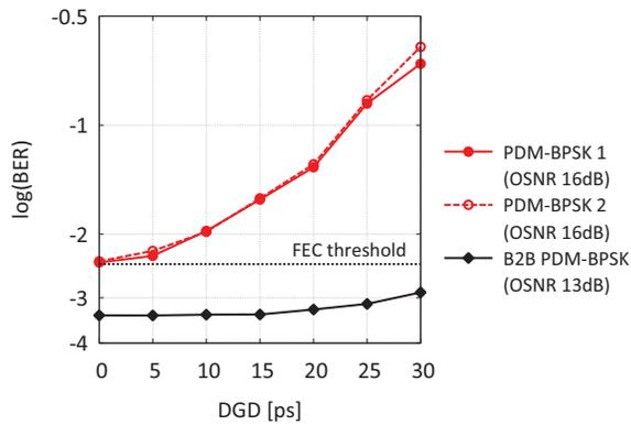
Fig. 12. BER as a function of DGD with emulated PMD effects on the original PDM signal.
