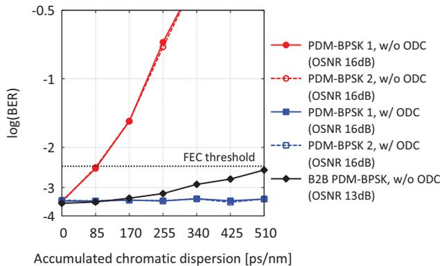
Fig. 10. BER as a function of chromatic dispersion accumulated before format conversion.
