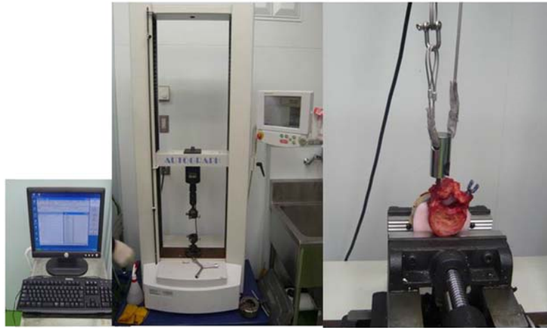
Figure 3 Screw pullout testing. A special adaptor was made to fit around the head of the pedicle screw.
