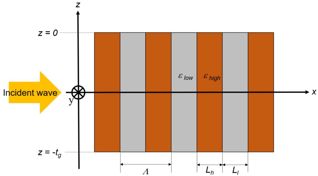
Figure 2.10 schematic diagram of 1D-PhC
