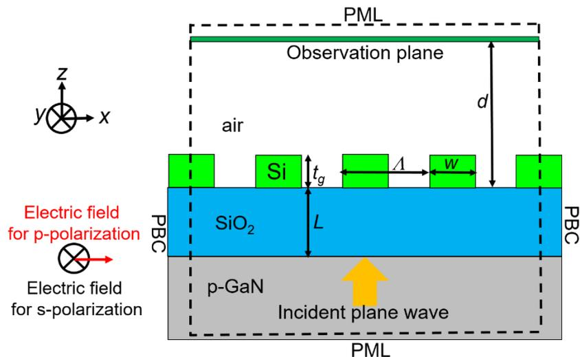
Figure 5.2 Numerical model of UV-LED with a SWG/SiO<sub>2</sub> underlayer
