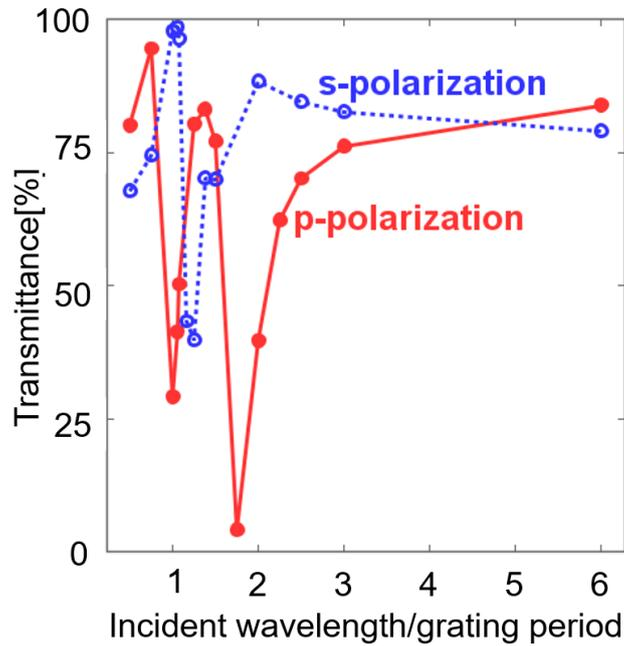
Figure 4.7 Dependence of the transmittance through the SWG on the grating period and polarization
