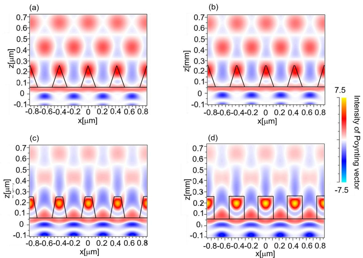
Figure 6.3 Poynting vector distribution at a certain time for s-polarization
