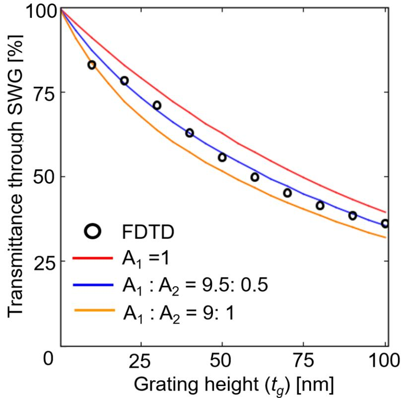
Figure 3.5 Dependence of  $p$ -polarization transmittance through Ge-SWG as a function of  $t_g$  for various 1st- and 2nd-order mode weights
