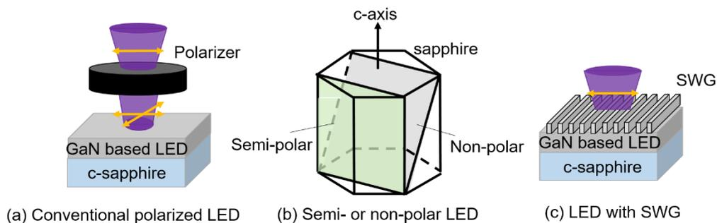
Figure 1.3 various types of GaN-based polarized LED structure
