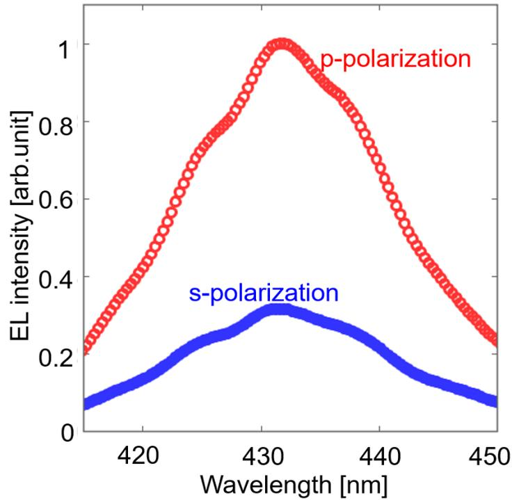
Figure 6.6 EL spectra of the emission from the LED with a trapezoid  $\text{SiO}_2$ -SWG
