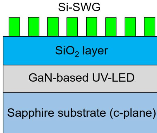
Figure 5.1 Schematic diagram of a UV-LED with a Si-SWG/SiO<sub>2</sub> underlayer structure
