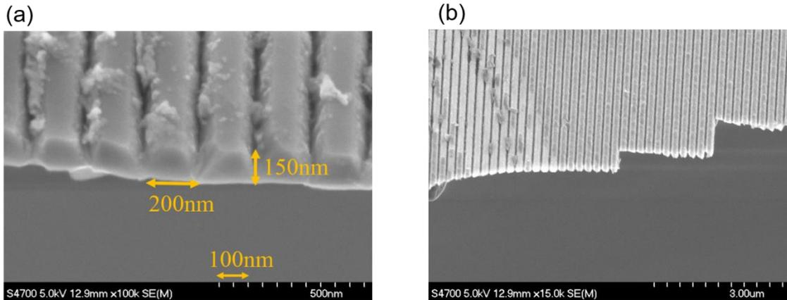
Figure 4.2 Cross-sectional view of the SWG fabricated on the top of conventional c-plane GaN-based UV-LED (a) 10000-, (b) 15000- magnification
