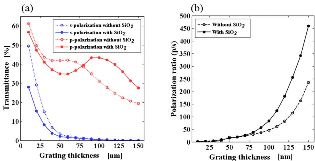
Figure 5.3 (a) Transmittance and (b) polarization ratio for the Si-SWG with and without the SiO<sub>2</sub> underlayer
