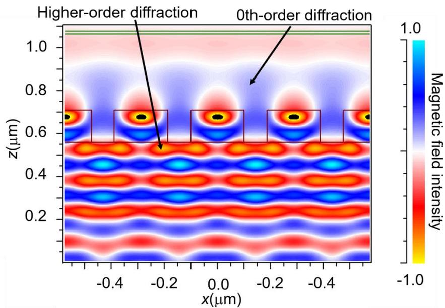
Figure 4.11 Magnetic field distribution of the SWG in the FDTD asymmetric model  $\lambda/\Lambda = 1.75$
