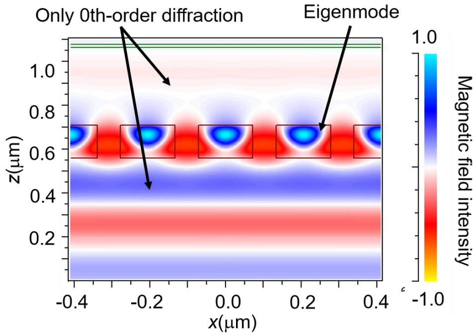
Figure 4.8 Magnetic field distribution within the SWG
