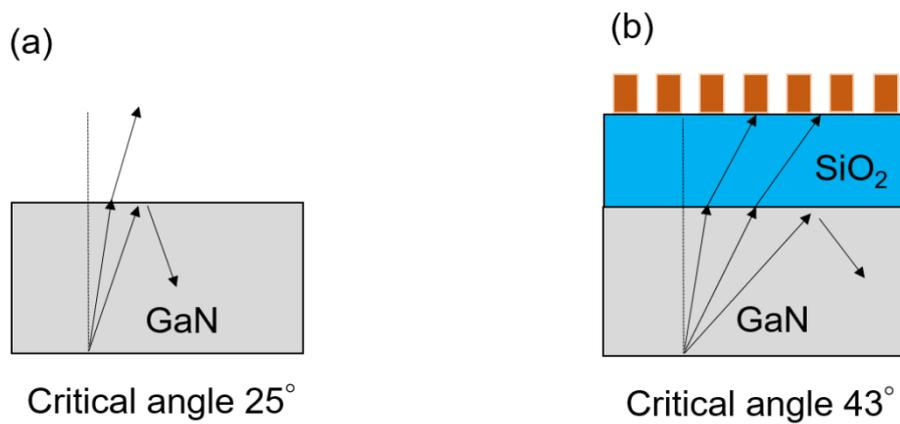
Figure 5. 10 Critical angle at (a) at GaN/air, (b) SiO<sub>2</sub>/GaN interface
