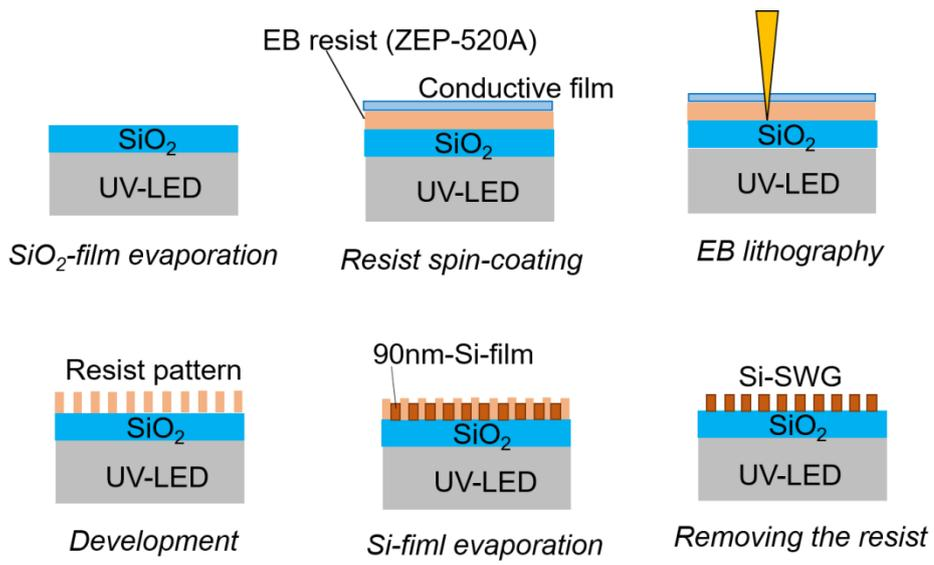
Fig. 5.5 Fabrication process of Si-SWG/SiO<sub>2</sub> underlayer
