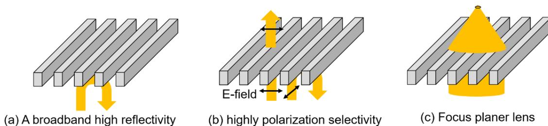
*Figure 1.2 Extraordinary properties of high contrast SWG structure*
