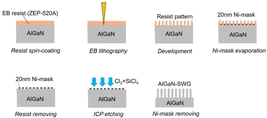
Figure 4.1 Fabrication processes of the SWG on the UV-LED
