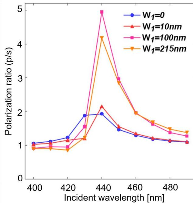
Figure 6.2 The  $\text{SiO}_2$ -SWG polarization ratio as a function of the incident light wavelength with  $W_1 = 0, 10, 100, \text{ and } 215 \text{ nm}$ .
