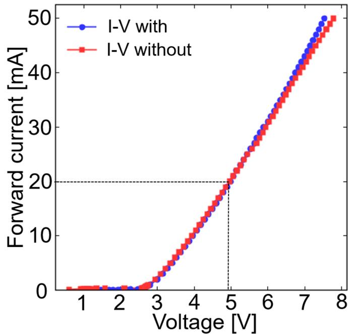
Figure 5.13 I-V characteristics of the GaN-based UV-LED without and with the Si-SWG/SiO<sub>2</sub> structure
