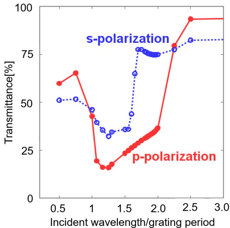
Figure 4.10 Dependence of the SWG transmittance on the grating period and polarization states
