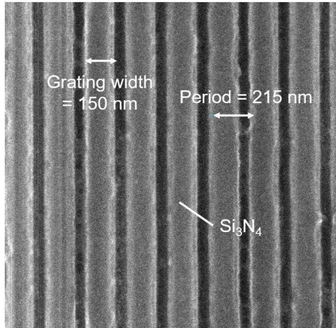
Figure 7.7 Top of image of the fabricated the Si<sub>3</sub>N<sub>4</sub>-SWG
