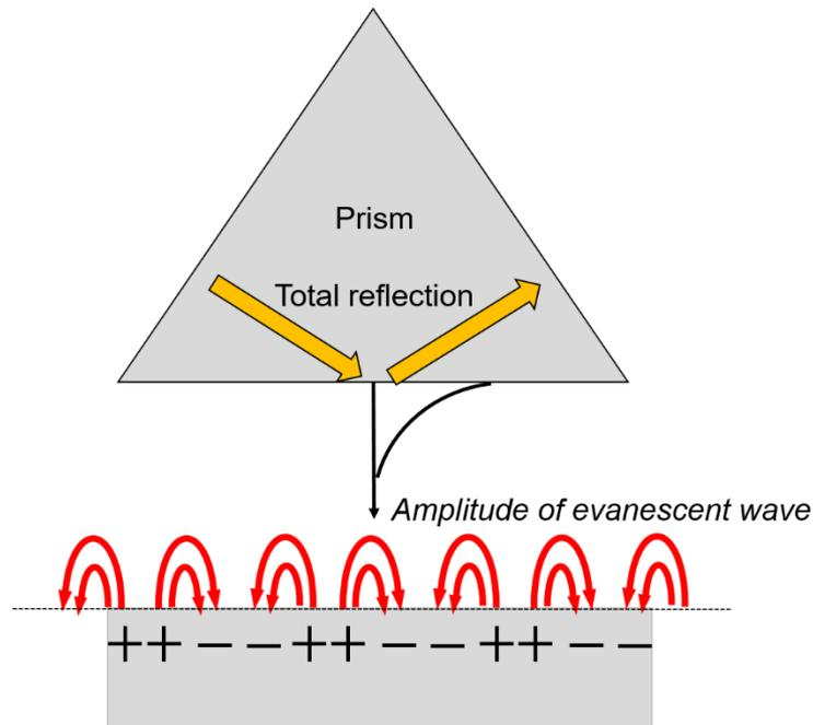
Figure 2.4 Cross section coupling of SP mode with the evanescent wave
