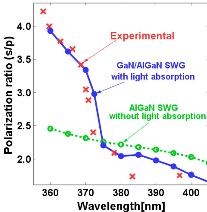
Figure 4.13 Dependence of the SWG polarization characteristics on the incident wavelength
