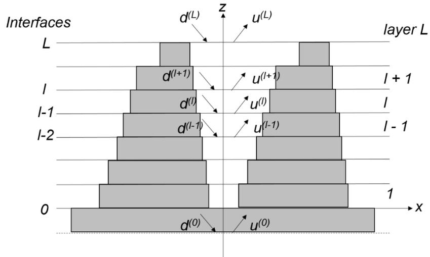
Figure 2.15 Optional shape structure model in RCWA simulation
