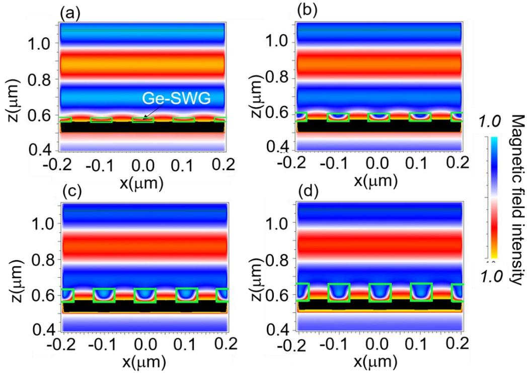
Fig. 3.4 Dependence of p-polarized eigenmode magnetic field distribution within Ge-SWG on  $t_g$ , for  $t_g =$  (a) 25, (b) 50, (c) 75, and (d) 100 nm
