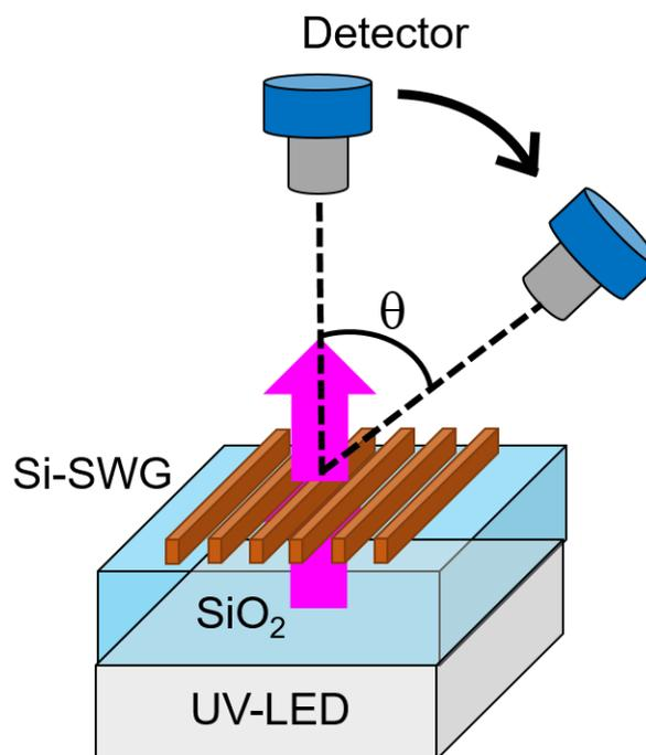
*Fig. 5.7 Measurement system of the angular dependence of the emission.*
