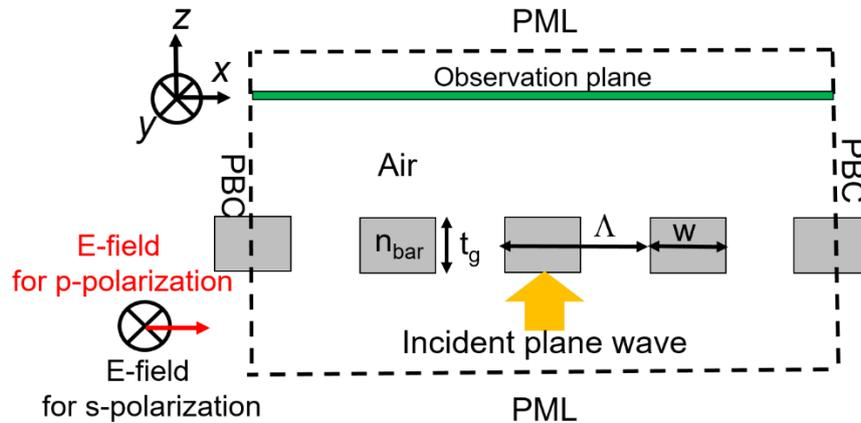
Figure 3.2 Cross-section of the FDTD calculation model.
