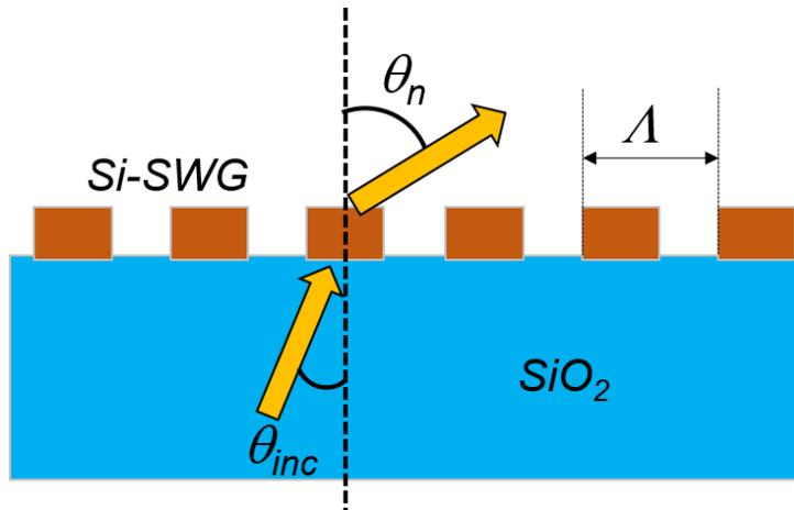
Figure 5.12 Cross section of Si-SWG/SiO<sub>2</sub>
