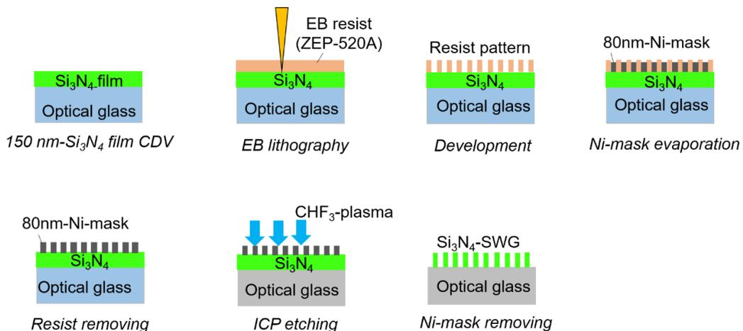
Figure 7.6 Fabrication processes of the  $Si_3N_4$ -SWG on the optical glass
