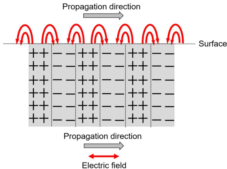
Figure 2.2 Schematic diagram of surface plasmon
