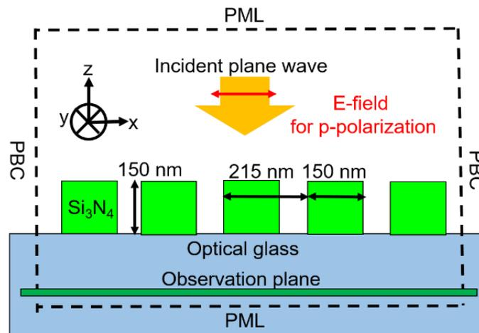
Figure 7.3 FDTD calculation model for the refractive index detection using Si<sub>3</sub>N<sub>4</sub>-SWG
