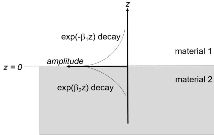
Figure 2.3 Field of the surface boundary mode
