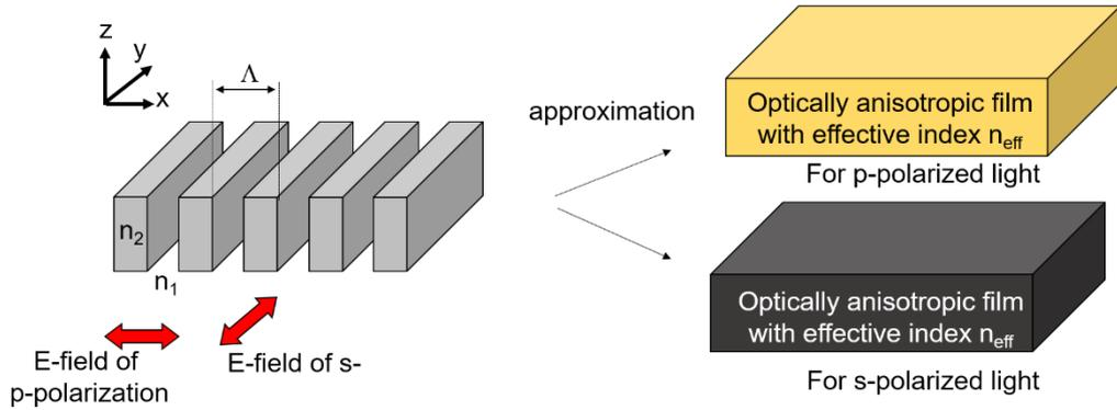
Figure 2.12 Schematic diagram of the EMT model
