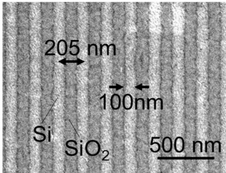
Figure 5.6 Top of view of the fabricated Si-SWG/SiO<sub>2</sub> underlayer
