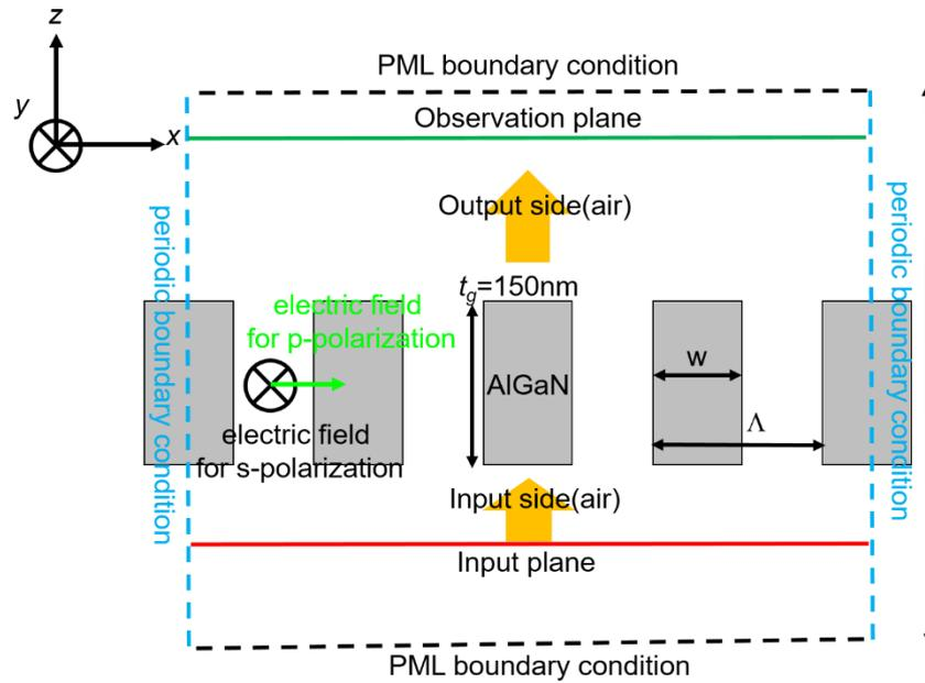
Figure 4.6 Schematic of the symmetric model in field simulation using FDTD method
