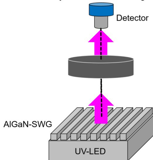
Figure 4.3 Experimental setup of EL emission measurement
