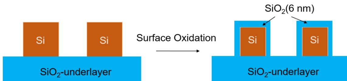
*Figure 5.9 Surface oxidation model of the Si-SWG*
