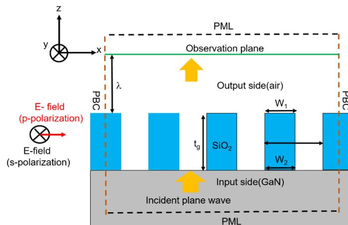
Figure 6.1 Numerical model for investigating electromagnetic field distribution.
