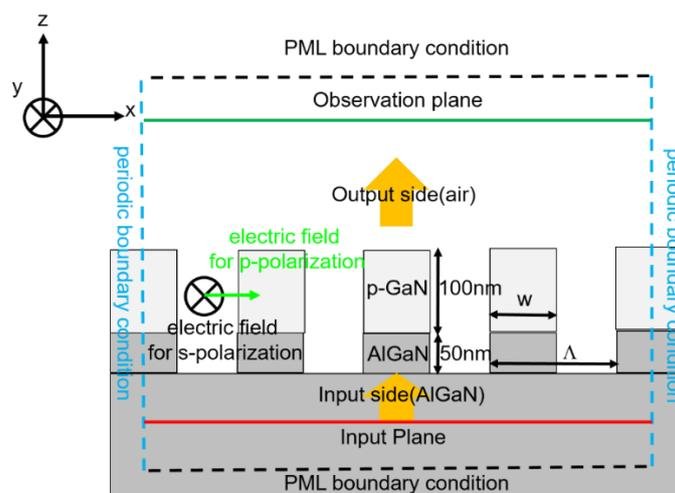
Figure 4.12 FDTD asymmetric model with 100 nm p-type GaN
