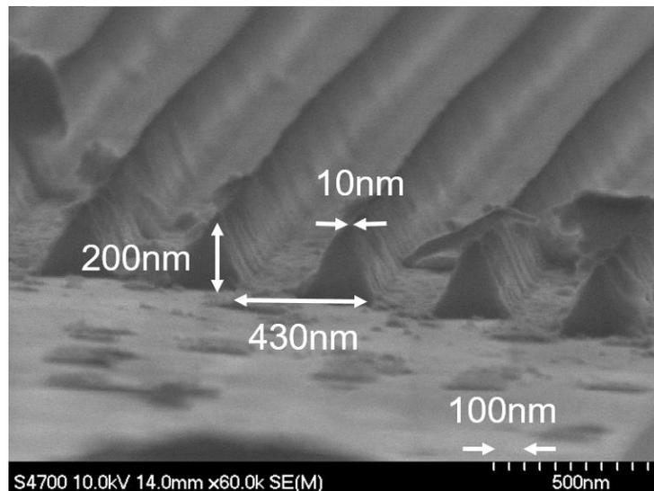
*Figure 6.5 Cross-sectional scanning electron microscope view of the SiO<sub>2</sub>-SWG fabricated on an InGaN-based LED.*
