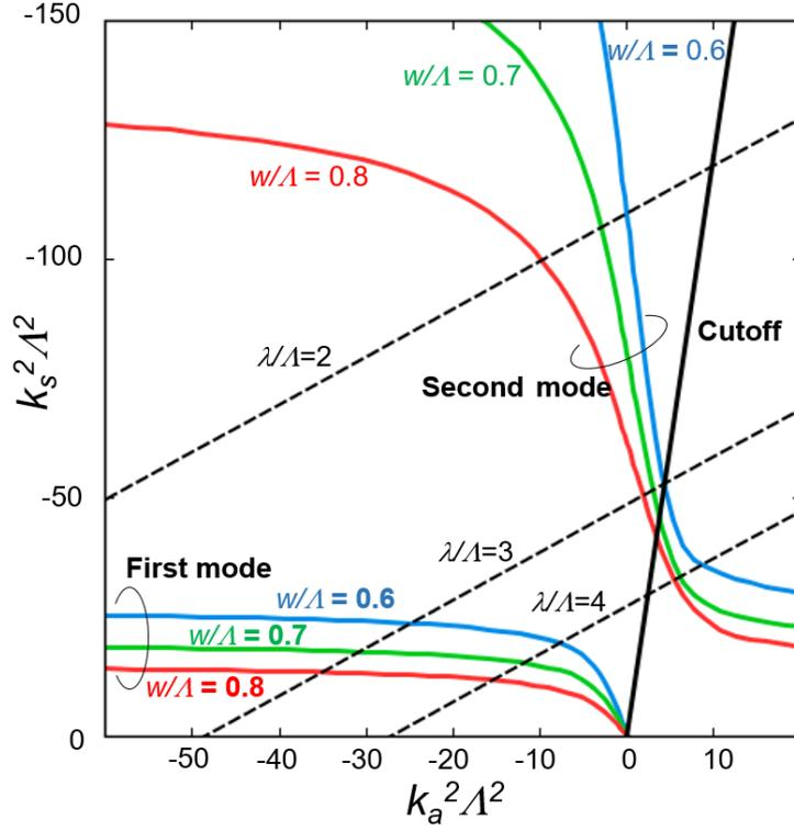
Figure 2.9 Dispersion relation between  $k_a$  and  $k_s$  in the SWG with  $n_{bar} = 3.48$  for  $p$ -polarized incidence. This dispersion relation is calculated by author referring [47]
