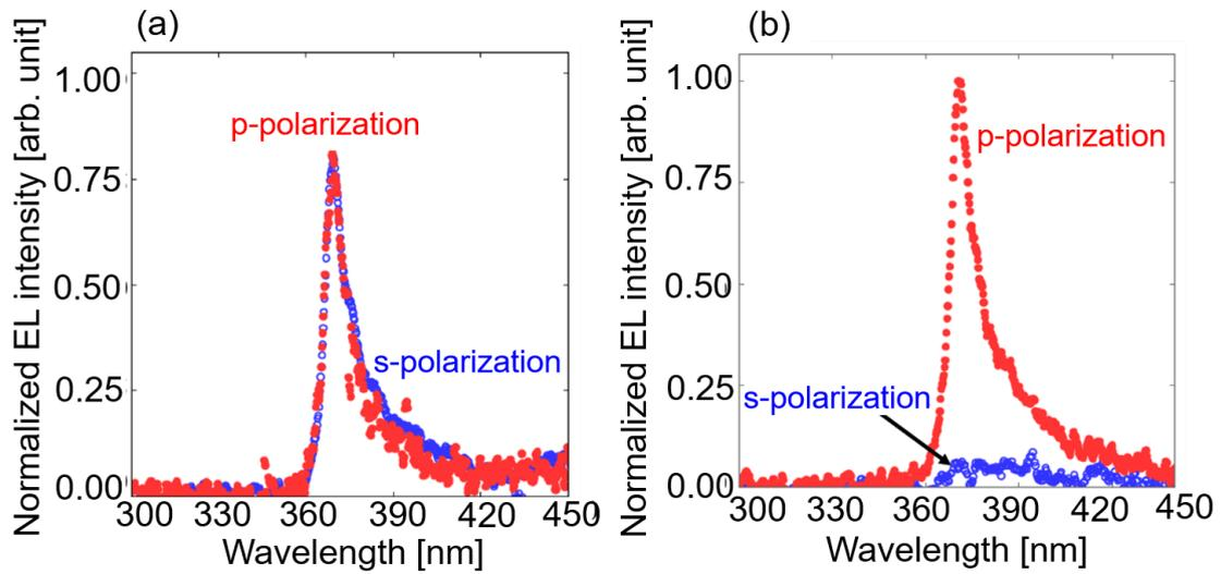
Figure 5.8 Normalized EL spectra for a forward current of 20 mA from the UV-LED, (a) without (b) with the Si-SWG/SiO<sub>2</sub> underlayer structure
