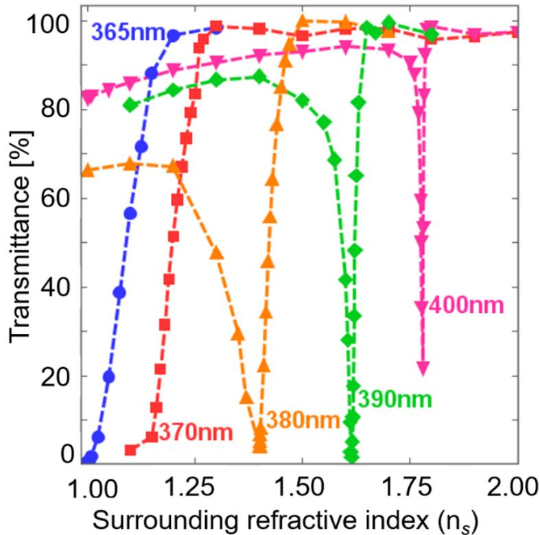
Figure 7.4 The FDTD calculated dependence of the transmittance on  $n_s$
