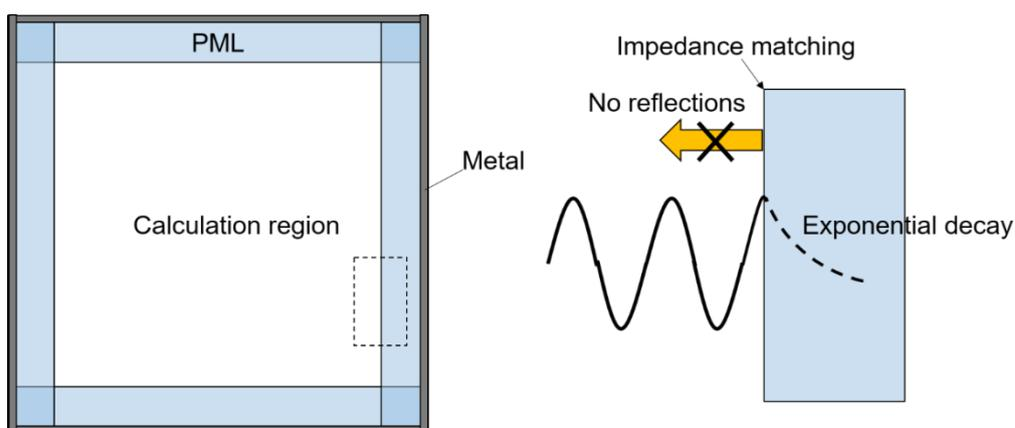
Fig. 2.17 Behavior of light wave in the PML
