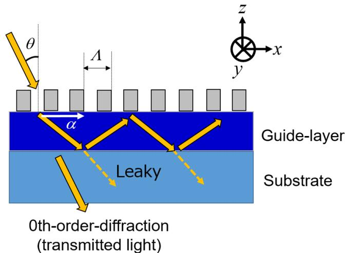
Figure 2.7 Geometry of GMR filter
