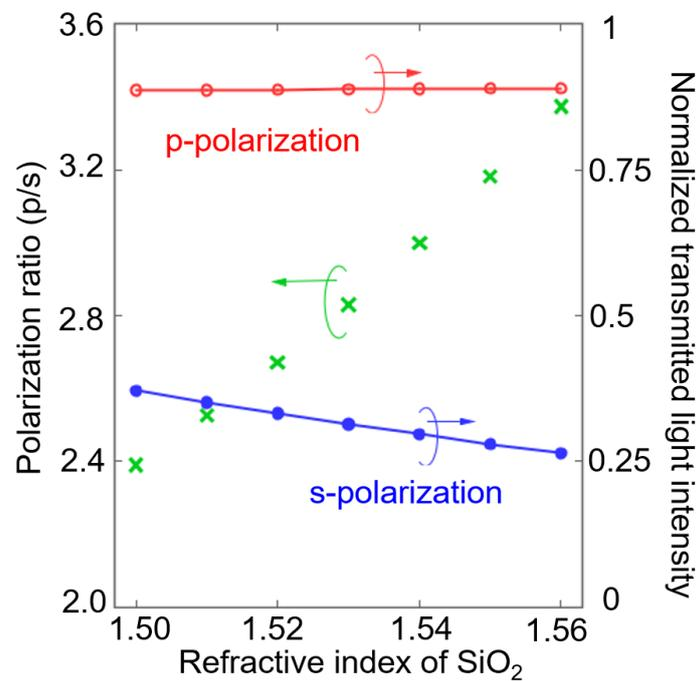
Figure 6.7 Dependence of the polarization characteristics of the emission on  $n_{\text{SiO}_2}$  at wavelength of 440 nm
