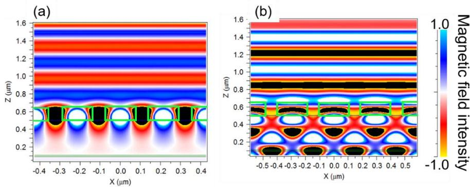
Figure 7.5 Magnetic field distribution at (a) low (b) high transmittance condition
