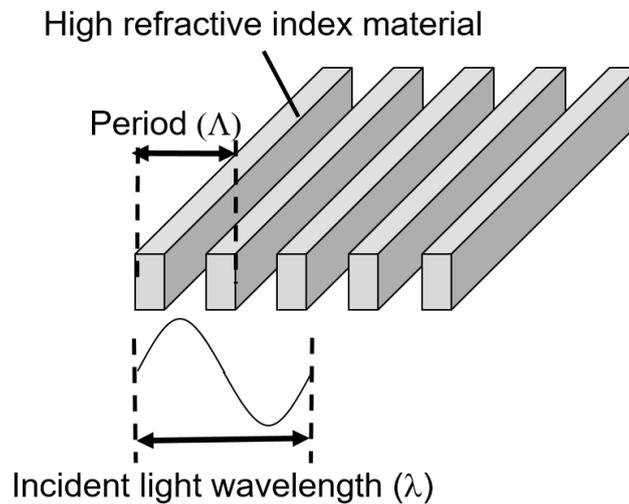
*Figure 1.1 Schematic diagram of a high contrast SWG*
