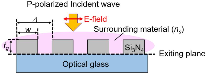
Figure 7.1  $\text{Si}_3\text{N}_4$ -SWG model for refractive index detection
