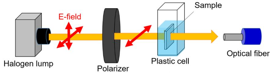
Figure 7.8 Experimental setup for the refractive index detection
