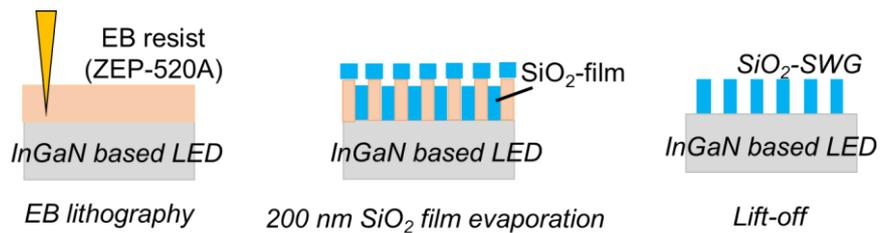
Figure 6.4 Fabrication processes of SiO<sub>2</sub>-SWG
