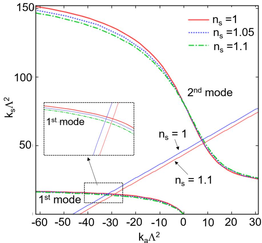
Figure 7.2 Wavenumber dispersion relation in  $\text{Si}_3\text{N}_4$ -SWG surrounded with  $n_s$
