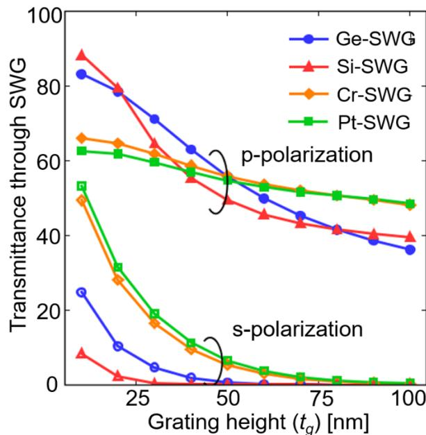
Fig. 3.3 Calculation of transmittance through SWG as a function of grating height ( $t_g$ )
