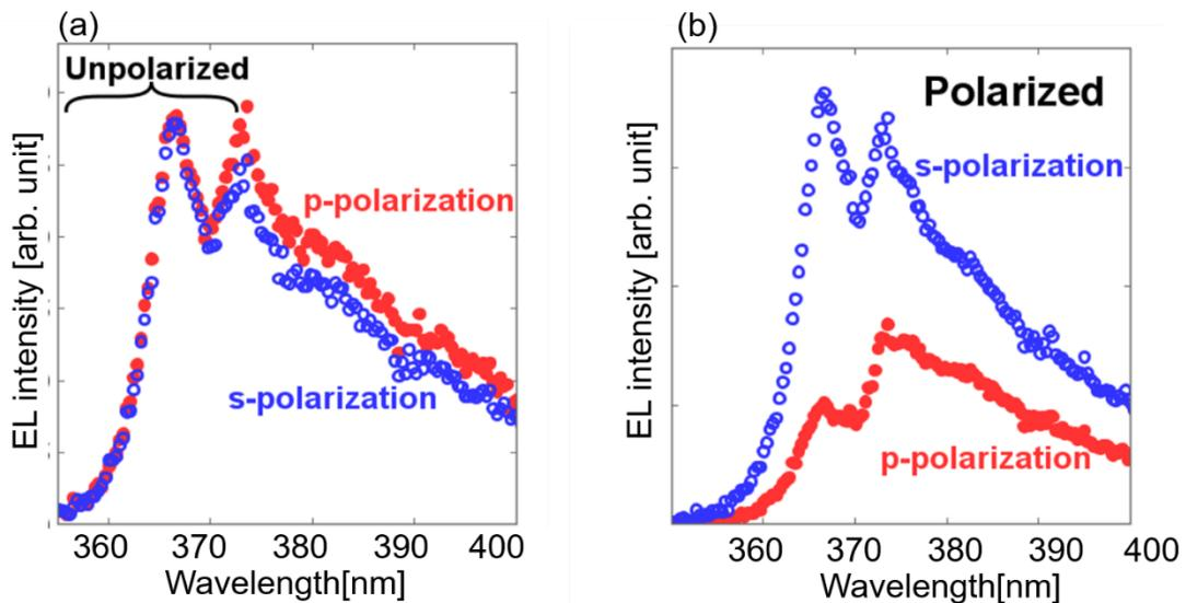
Figure 4.4 Emission spectra from UV-LED: (a) without (b) with the SWG structure at a forward current 20mA
