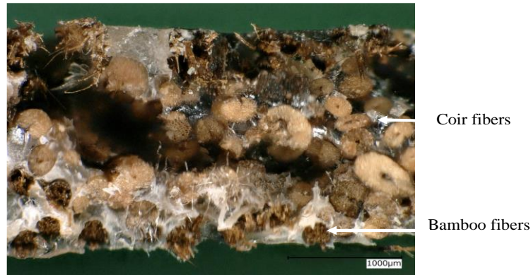
Figure 5.7 Optical microscopy images of fracture surfaces of untreated bamboo and coir fibers embedded in PLA in BCCB/PLA.
