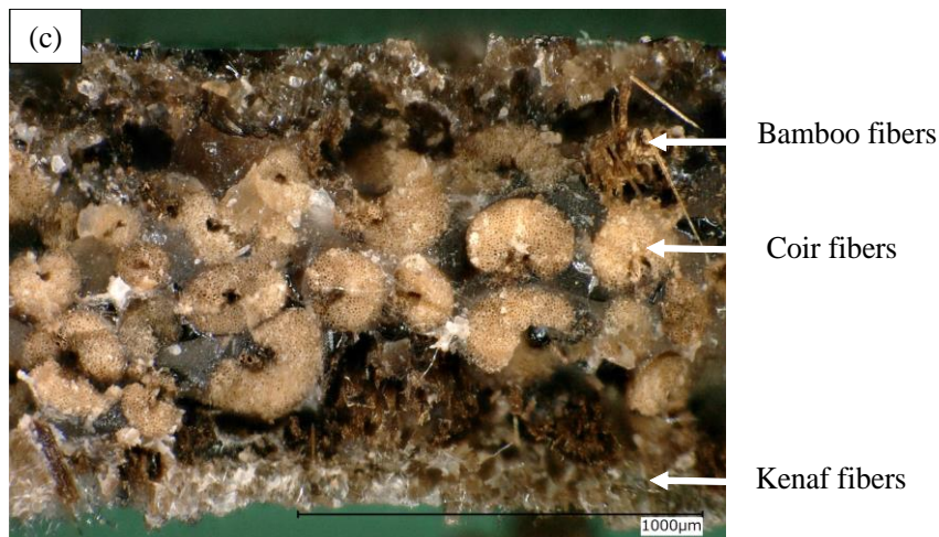
Figure 5.11 Optical microscopy images of fracture surfaces of untreated kenaf, bamboo and coir fibers embedded in PLA in KBCCBK/PLA.
