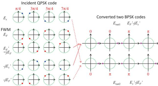
**Fig. 2** Constellation of each incident QPSK code and the converted BPSK codes.
