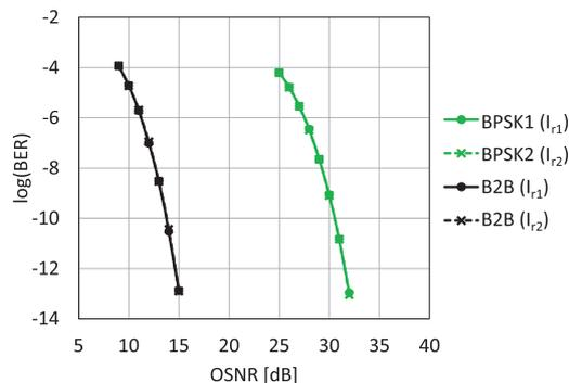
**Fig. 7** BER performance of the format conversion for NRZ signals using 100-m HNLF, where the pump power is 10 dBm, and the signal power is 6.56 dBm at the WDM combiner.
