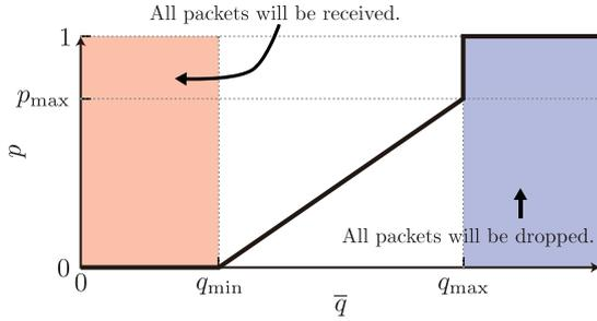
**Fig. 1** Structure of the drop probability of a packet. When  $\bar{q}$  is less than  $q_{\min}$ ,  $p$  is set for zero, thus all packets will be received without loss of packets.
