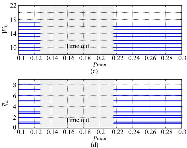
**Fig. 6** One-dimensional bifurcation diagram varied the parameter  $p_{\max}$  on the line (ii) in Fig. 4. ( $w_q = 0.13$ ) (y-axis: the window size  $W_k$  and the average queue size  $\bar{q}_k$  [packets]).
