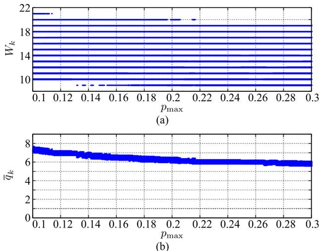
**Fig. 5** One-dimensional bifurcation diagram varied the parameter  $p_{\max}$  on the line (i) in Fig. 4. ( $w_q = 0.002$ ) (y-axis: the window size  $W_k$  and the average queue size  $\bar{q}_k$  [packets]).
