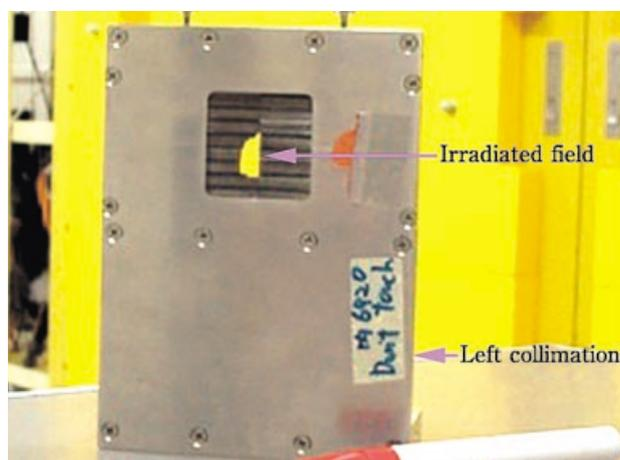
Fig. 1. The rat left hemisphere was irradiated with HIMAC (Heavy Ion Medical Accelerator in Chiba), and its irradiated field (above arrow) was confirmed with this left collimation which was made of lead.
