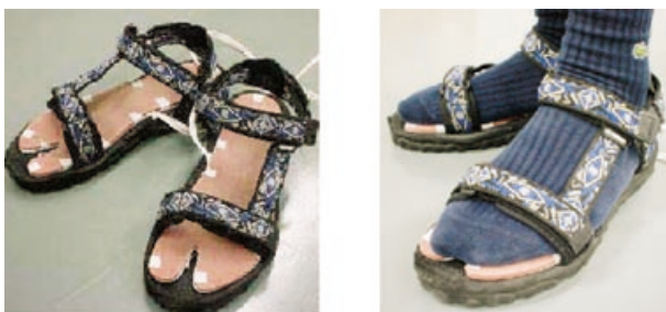
Fig. 10. Heel-to-toe pressure sensors
