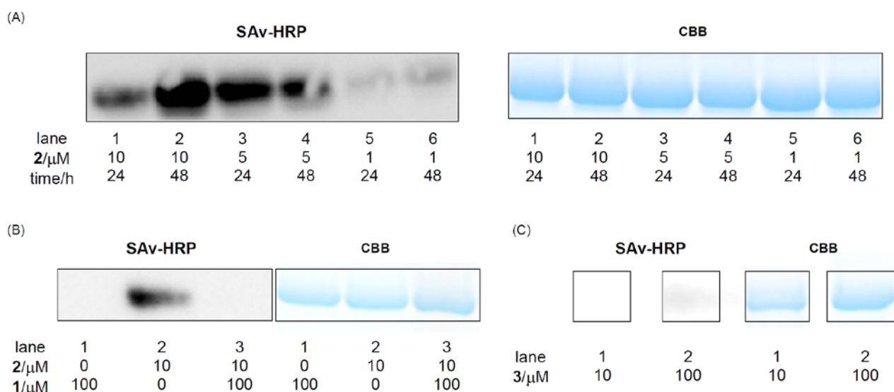
Fig. 4 SDS-PAGE analyses for the labeling of hDAO with the SEAL reagent. (A) hDAO (10 \mu\text{M} ) with stabilizers (1 \mu\text{M} FAD, 10 \mu\text{M} dithiothreitol, 20 \mu\text{M} sodium benzoate, 5 mM KCl) was incubated with SEAL reagent 2 (10, 5 or 1 \mu\text{M} ) in Tris buffer (50 mM, pH 8.3) at 37 ^\circ\text{C} for 24 or 48 h. (B) hDAO (10 \mu\text{M} ) with stabilizers (1 \mu\text{M} FAD, 10 \mu\text{M} dithiothreitol, 20 \mu\text{M} sodium benzoate, 5 mM KCl) was incubated with SEAL reagent 2 and/or inhibitor 11 in Tris buffer (50 mM, pH 8.3) at 37 ^\circ\text{C} for 48 h. (C) hDAO (10 \mu\text{M} ) with stabilizers (1 \mu\text{M} FAD, 10 \mu\text{M} dithiothreitol, 20 \mu\text{M} sodium benzoate, 5 mM KCl) was incubated with negative control 3 (10 or 100 \mu\text{M} ) at 37 ^\circ\text{C} for 48 h. An original picture of Fig. 4C before band separation is shown in Fig. S1 in ESI.
