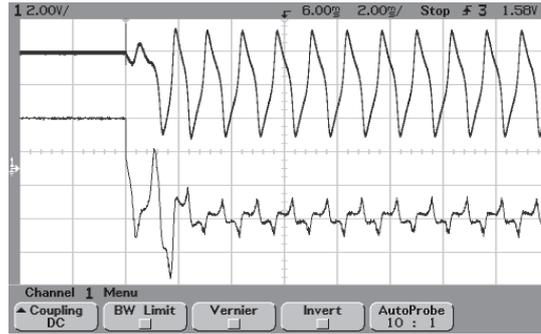
Fig. 13. Time responses of the control. The horizontal axis: 2 [msec/DIV]. Upper: Capacitor voltage corresponding to  $x$  in Eqs. (7) with the vertical axis: 2[V/div]. Lower: Injection current corresponding to the control input with the vertical axis: 0.2 [mA/div].
