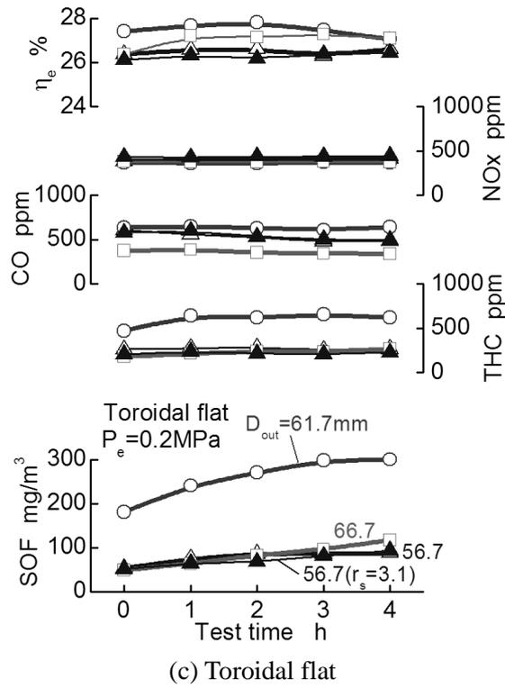
**Fig.4.** Change in exhaust emissions. (a) R35. (b) R45. (c) Toroidal flat.
