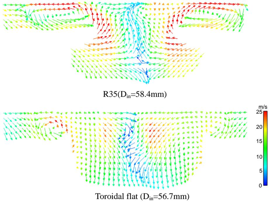
**Fig.9.** Analysis of gas flow (31° ATDC).
