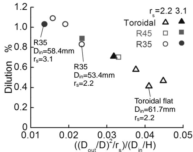
**Fig.12.** Effect of gas flow on fuel dilution.
