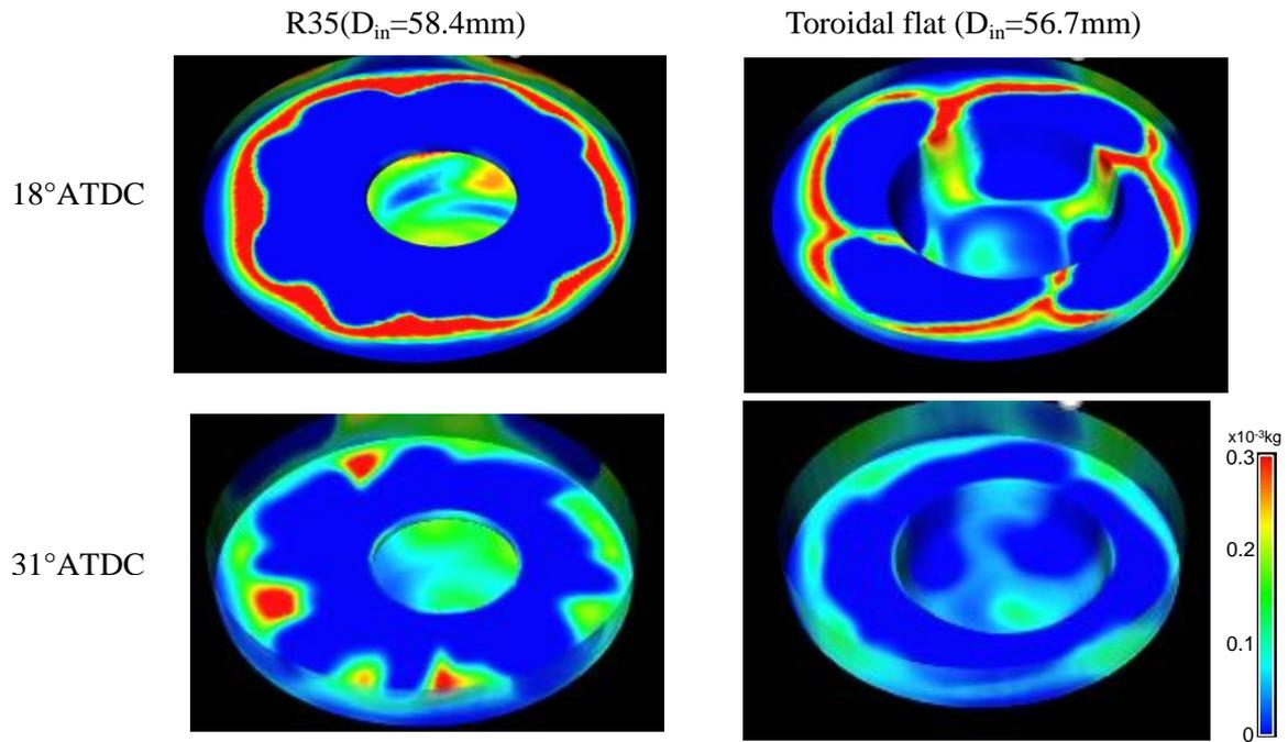
**Fig.7.** CFD analysis of fuel distribution near the top surface of piston.
