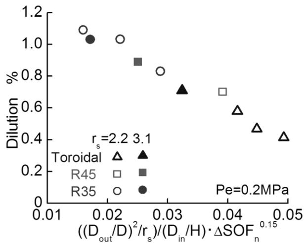
**Fig.15.** Effect of gas flow parameters and SOF emission on fuel dilution.
