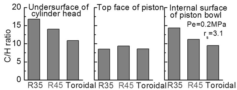
**Fig.8.** Elementary analysis (C/H ratio) of deposit.
