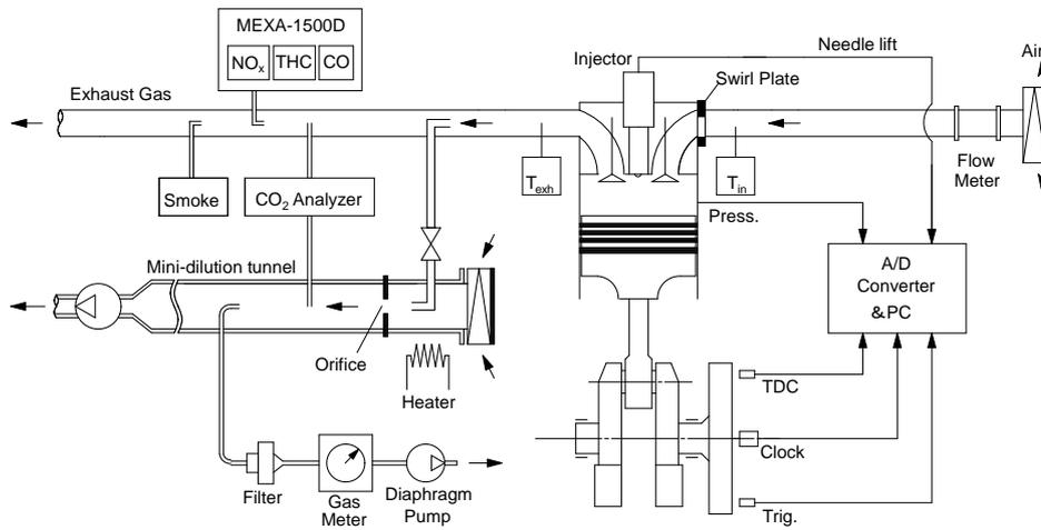
**Fig.2.** Experimental setup.
