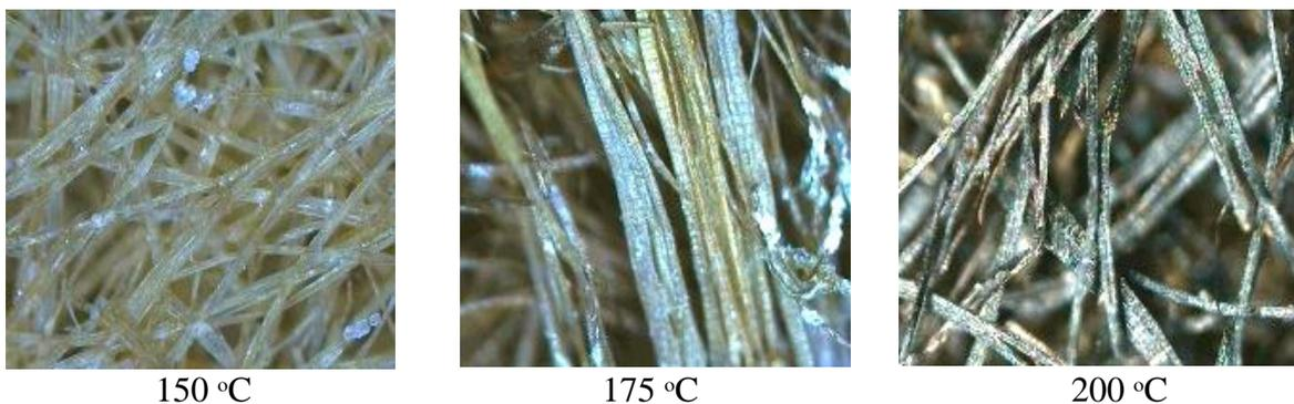
Figure 4.10: KF-IZO appearances after different annealed temperature (MORITEX – Scopemen series with 166× magnification).
