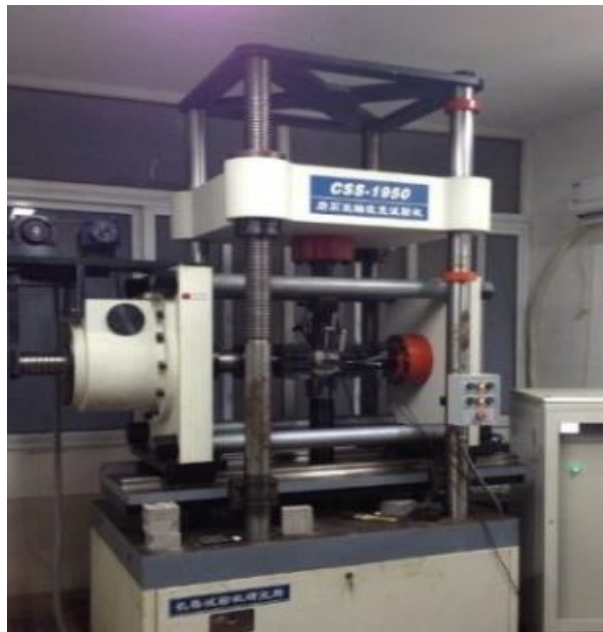
Figure 2.4 CSS-1950 biaxial shear rheological testing equipment
