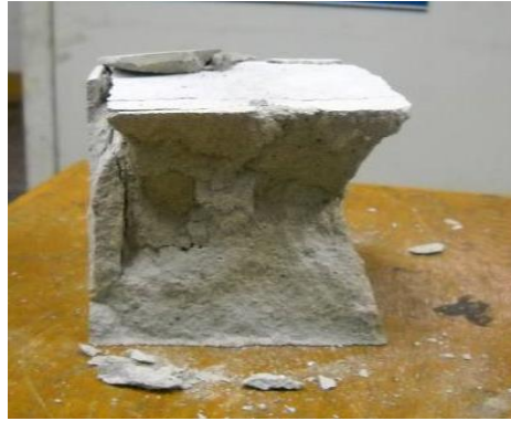
Figure 2.5 Typical failure pattern of intact samples
