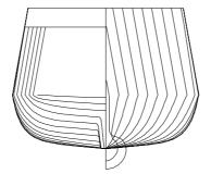
Fig.2 Body plan of the ONR tumblehome vessel.
