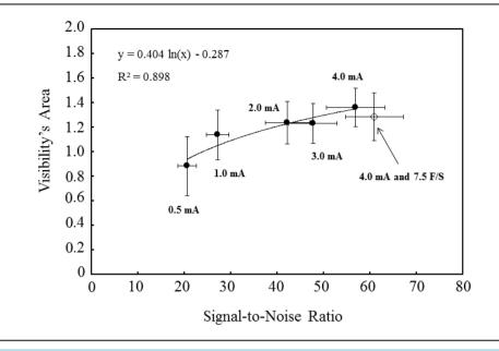
Figure 7. Relationship between signal-to-noise ratio and visibility.
