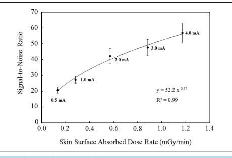
Figure 4. Signal-to-noise ratio for skin surface absorbed dose rate.
