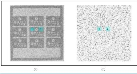
Figure 3. Two regions of interest on the static image: (a) For signal data; (b) For noise data.
