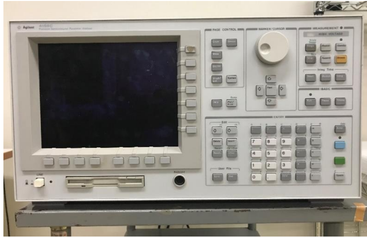
Fig.5 Photograph of I - V measurement instrument of Agilent 4156C.
