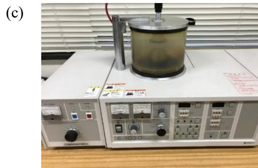
Fig. 36 (a) shows the process of graphene sample etching. (b) Graphene sample patterned design. (c) is the etching equipment E -1030 HITACHI ion sputter for this experiment.
