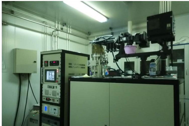
Figure 2-1 Picture of the AX5200 MPCVD system used for diamond growth.
