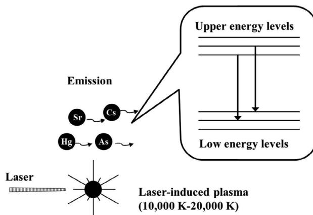
Fig. 1. LIBS plasma process.
