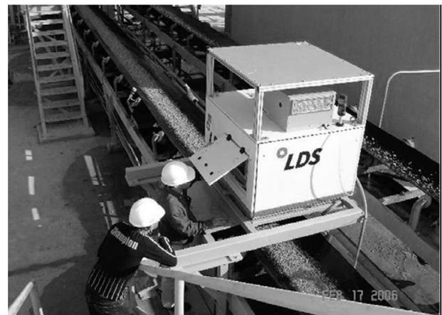
**Fig. 6.** On-line monitoring in iron making processes<sup>32)</sup> “Reprinted with permission from (M. Gaft, I. Sapir-Sofer, H. Modiano and R. Stana: Laser induced breakdown spectroscopy for bulk minerals online analyses. *Spectrochimica Acta Part B: Atomic Spectroscopy*. 2007; 62, 1496–1503. DOI:10.1016/j.sab.2007.10.041). Copyright (2007) Elsevier”.
