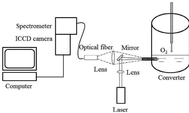
Fig. 8. Concept of LIBS application to a decarburization converter.
