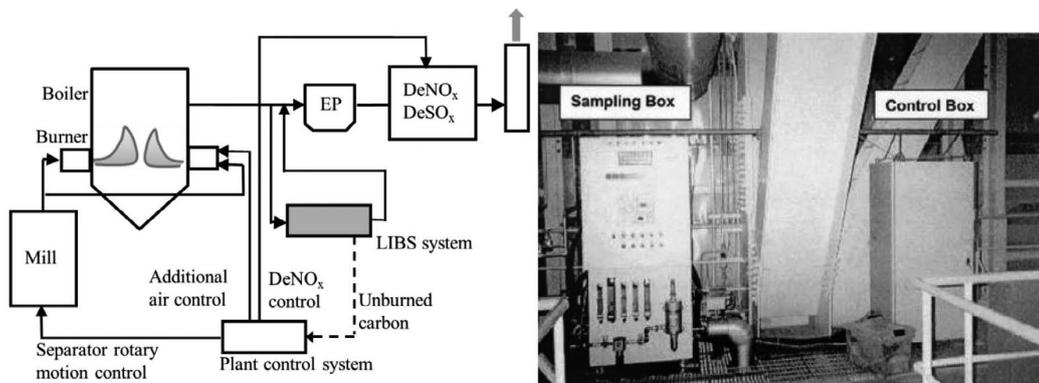
(a) Optimal boiler control system. (b) Photograph of unburned-carbon measurement apparatus.
