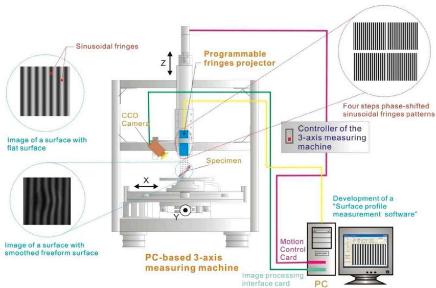
(a) Setup for the 4-step fringes projection system
