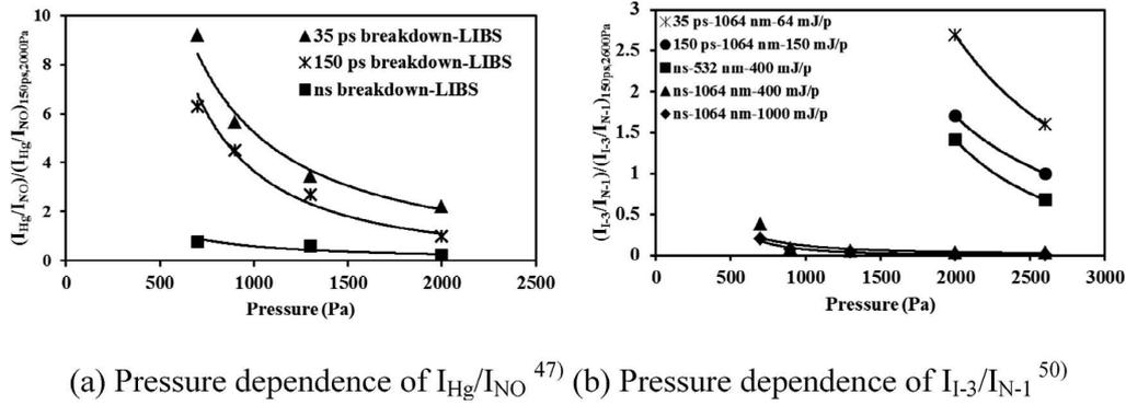
Fig. 4. Pressure dependence of the intensity ratios of  $I_{Hg}/I_{NO}$  and  $I_{I-3}/I_{N-1}$  under different conditions using LIBS.
