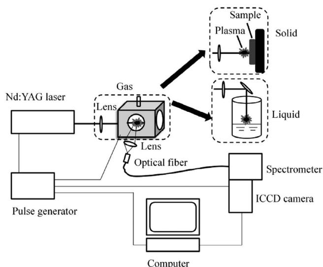
Fig. 2. Typical geometric arrangement of LIBS.
