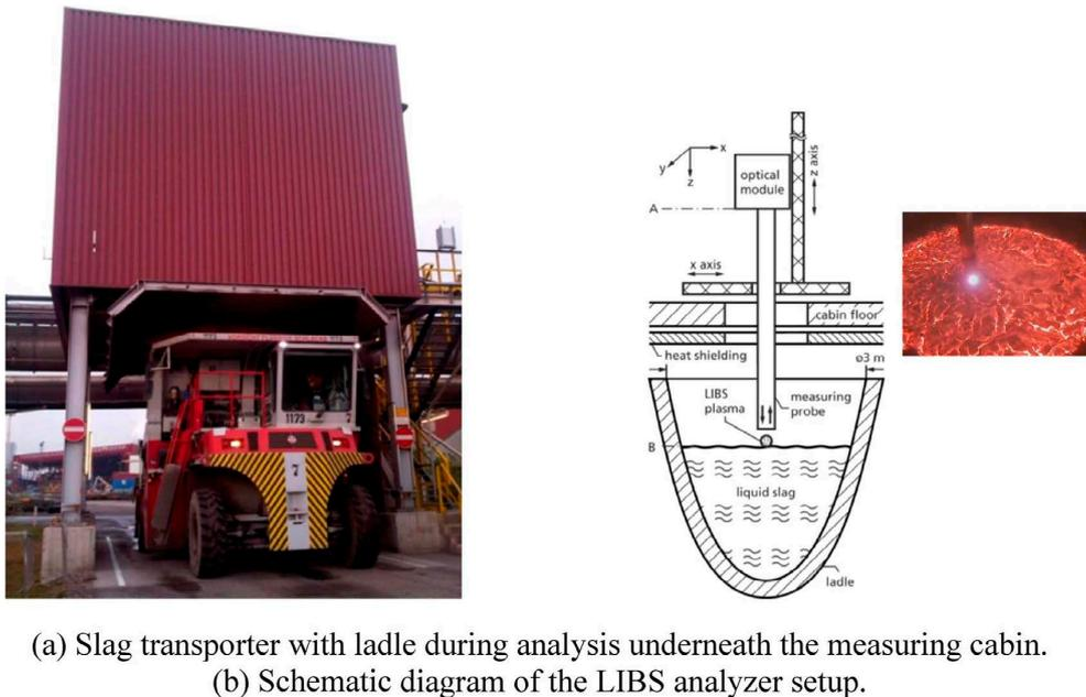
**Fig. 11.** Application of LIBS in liquid slag analysis<sup>106)</sup> “Reprinted with permission from (V. Sturm, R. Fleige, M. de Kanter, R. Leitner, K. Pilz, D. Fischer, G. Hubmer, and R. Noll: Laser-Induced Breakdown Spectroscopy for 24/7 Automatic Liquid Slag Analysis at a Steel Works. *Analytical Chemistry*. 2014; 86, 9687–9692. DOI: 10.1021/ac5022425). Copyright (2014) American Chemical Society”. (Online version in color.)
