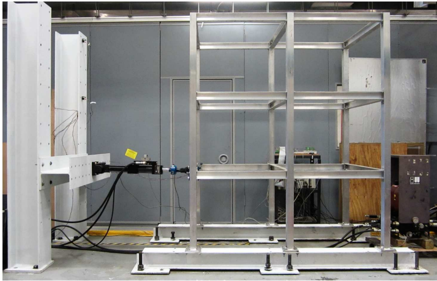
Figure 12. Picture of the 1:5 scaled model structure.
