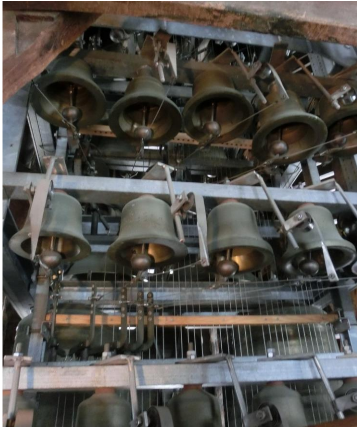
Figure 1: Musical instrument of Carillon with automatic play of multiple bells.
