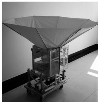
**Figure 12.** The prototype of winter jujube harvesting and sorting device.
