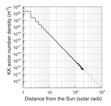
**Fig. 1.** Number density of trapped KK axions against the distance from the Sun. The black solid histogram shows the simulated distribution taken from Ref. [8] with  $g_{a\gamma\gamma} = 9.2 \times 10^{-14} \text{ GeV}^{-1}$ . The red dotted line shows the fitted  $r^{-4}$  curve. The unit of distance is the radius of the Sun (695,700 km). Using this unit, the distance between the Earth and the Sun is  $211.4R_{\odot}$  at perihelion and  $218.6R_{\odot}$  at aphelion.
