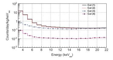
**Fig. 4.** Energy spectra of the observed data after each reduction step. The histogram with the black solid line shows the events after cut (1), the red dotted line shows the events after cut (2), the blue dash-dotted line represents the events after cut (3), and the magenta solid line with filled circle shows the events after cut (4), which is the final sample.
