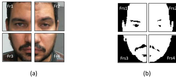
Fig. 5.2 The reference frame (a) The face detection and (b) The Skin-Color detection.
