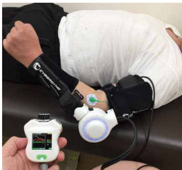
Fig 2. The single-joint Hybrid Assistive Limb(HAL-SJ). The controller showing the Bioelectrical signals.
