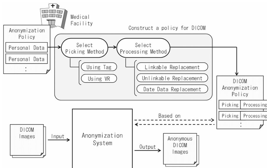
Fig. 2. Procedure of anonymization method.
