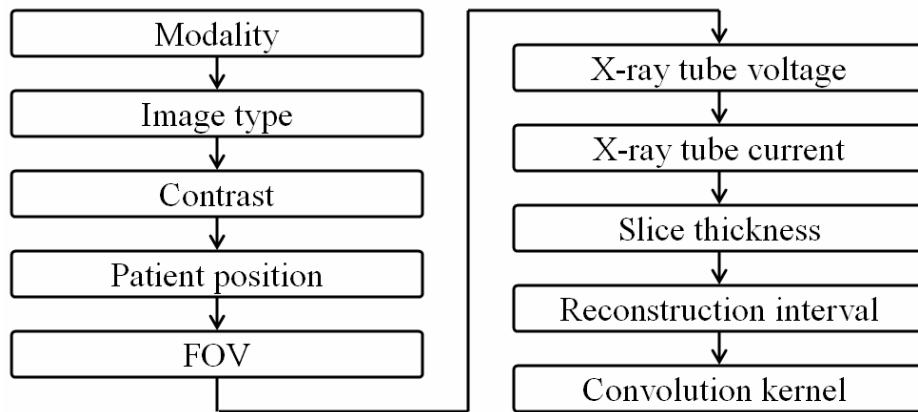
Fig.2. Procedure of distinction using textual meta information.
