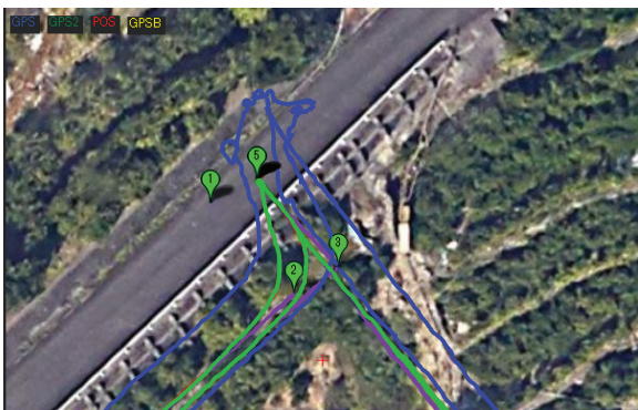
Fig. 11. Automatic navigation trajectory near the relay point.
