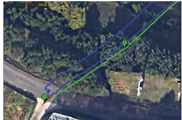
Fig. 12. Automatic navigation trajectory near the harvesting station.
