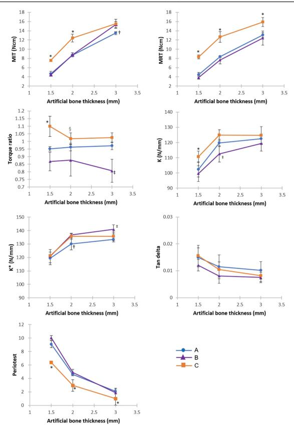
**Figure 2** Comparison of mechanical parameters among the three types miniscrews installed at artificial bone blocks with 1.5, 2.0 and 3.0 mm thickness (n = 5 for each thickness). \*p < 0.05 vs A and B with the same thickness;  ${}^{i}p < 0.05$  vs B and C with the same thickness;  ${}^{i}p < 0.05$  vs A and C with the same thickness;  ${}^{i}p < 0.05$  vs A and C with the same thickness;
