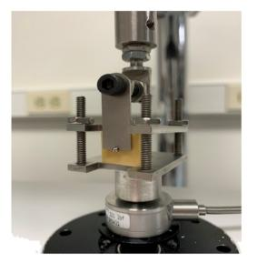
Figure 1 (a) Miniscrews installed at artificial bone with different thickness. (b) Experimental set-up for static and dynamic stiffness of the miniscrew system.
