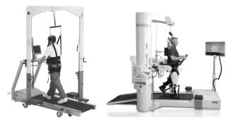
(a) AFO (hanging type).(b) LOKOMAT (Hocoma Co.).Fig. 1. Types of gait rehabilitation equipment.
