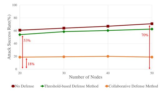
Figure 10: Attack success rate: Spy node assisted smart BH attack.
