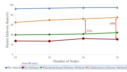
Figure 6: Packet delivery rate: Single smart BH node.
