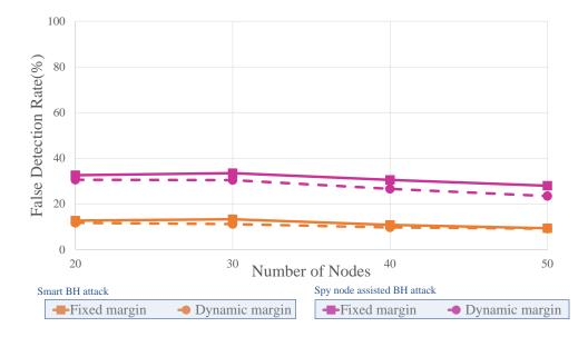
Figure 16: False detection rate: Single smart BH attack V.S. Spy node assisted smart BH attack.
