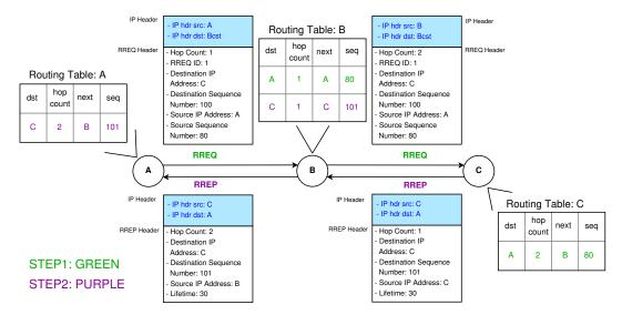
Figure 1: AODV: Route construction using RREQ and RREP.
