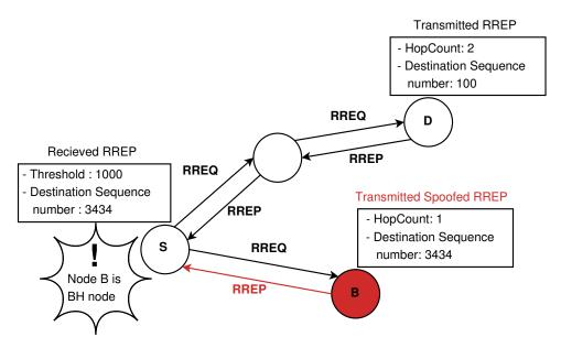
Figure 3: Threshold-based defense method.
