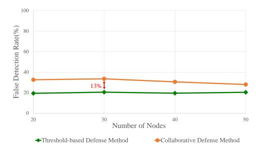
Figure 11: False detection rate: Spy node assisted smart BH attack.
