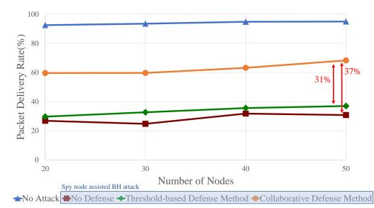
Figure 9: Packet delivery rate: Spy-node-assisted smart BH attack.
