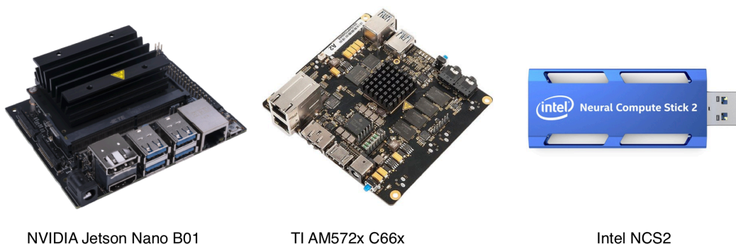
Figure 11: Three embedded systems used for our experiments. More and more vendors continue to show interest when it comes to deep learning on small form factors
