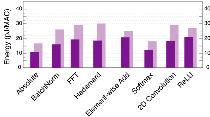
Figure 15: DSP accelerated algorithms show best overall results because of domain-specific environment for convolutions. In dark purple: Q-format with auto-differentiation. In light purple: the IEEE 754-2008 results under similar conditions.
