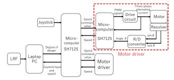
Figure 2: Hardware configuration of electric wheelchair
