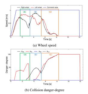
Figure 8: Transition of wheel speeds and degree of danger
