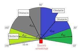
Figure 4: Definition of scanning area of LRF
