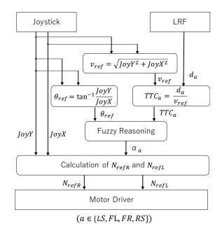
Figure 3: Safe driving support system
