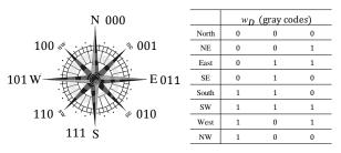
Figure 2: Definition of wind speed direction  $w_D(t)$
