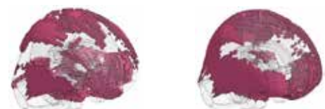
Fig 8. The finite elements those strain beyond the threshold by the 1st impact, in the case of Judo (left), American football (right).
