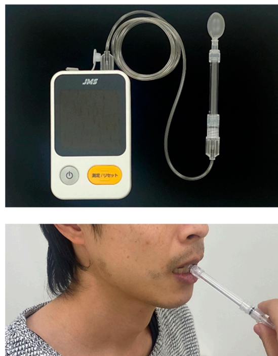
Figure 2. JMS tongue pressure measurement device (top), and measurements of tongue pressure (bottom).
