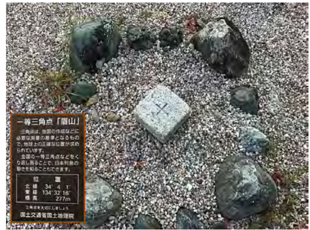
Fig. 10. Triangular point in the Tokushima prefecture, Japan.
