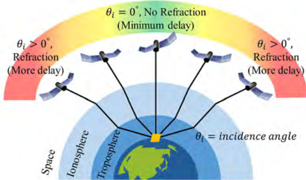
Fig. 2. Propagation delay by refraction on the ionospheric passage.
