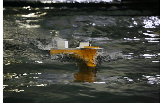
Fig. 17. Free-running model experiment.
